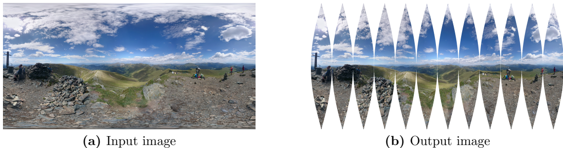
Figure 5.1: We use a tool to create sphere gores from cylindrical projections.
