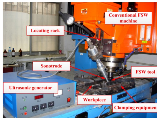
Fig. 1 The ultrasonic vibration enhanced friction stir welding (UVeFSW) system.
