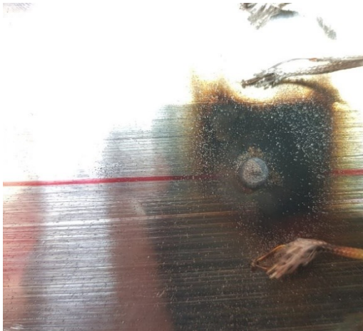
Fig. 6 unmolten particles on the surface of the test plate.
