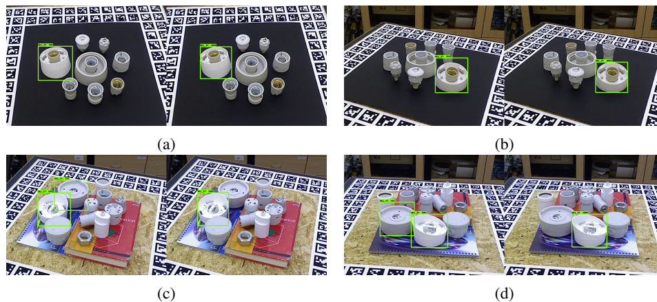
Fig. 6: Qualitative results of the texture-less object detection system. Each couple of images report the network detection (left) and the ground truth detection (right). (a) and (b) represents positive examples of detection, with high score in terms of accuracy in the detection and IoU ( Intersection over Union ) between network detection and ground truth. On the contrary (c) and (d) depict some examples of failures.
