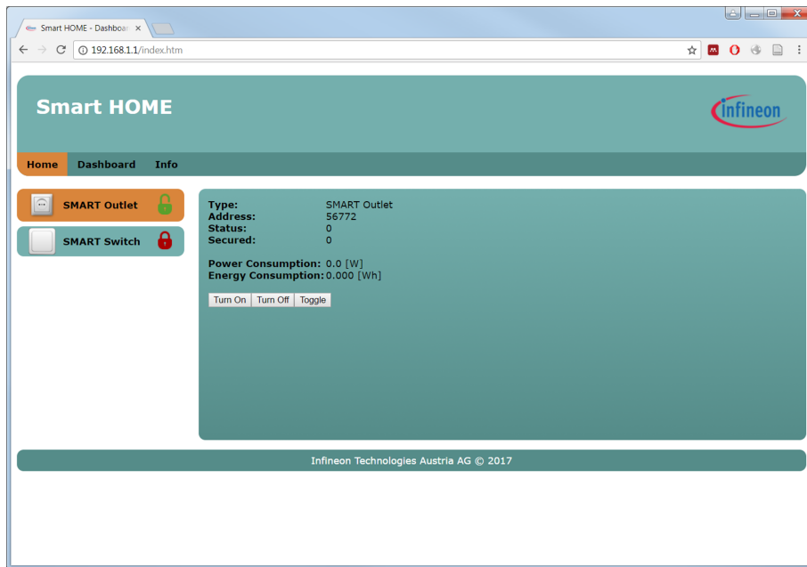
Figure 5.10: Website in “home” view with two connected IoT nodes, one smart switch, and one smart outlet. Left side shows the list of currently connected IoT nodes, and on the right side the detailed information of the selected node is illustrated.
