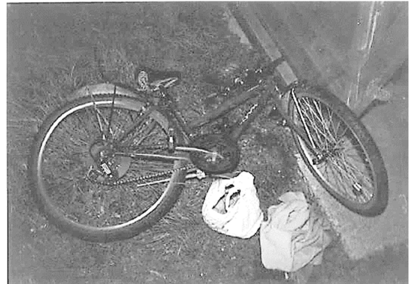
Figure 125: Damages to the bicycle from real-world case with left-turning bicyclist
