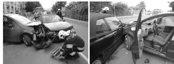
Figure 4: Two vehicles in the same crash scenario. One has the driver airbag inflated, in the other the driver airbag did not deploy (right). Image courtesy fire brigade.
