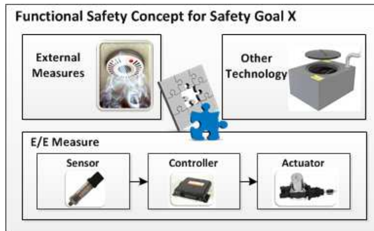
Fig. 7 Principle of Functional Safety Architecture consisting of three types of safety measures
