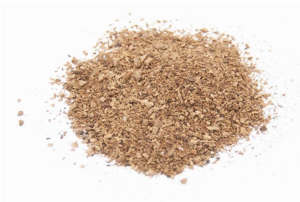
FIGURE 14: Picture of a typical pulp obtained under 210 °C for 3 h under 40 bar H 2 (Ex 6)
