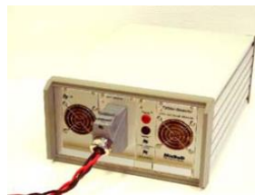
Figure 16: T3ster Booster – power switching unit [18]
