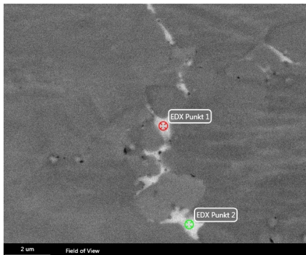
Figure 72: Filled crack of zinc-painted sample tested at 800°C showing the location of spot scans
