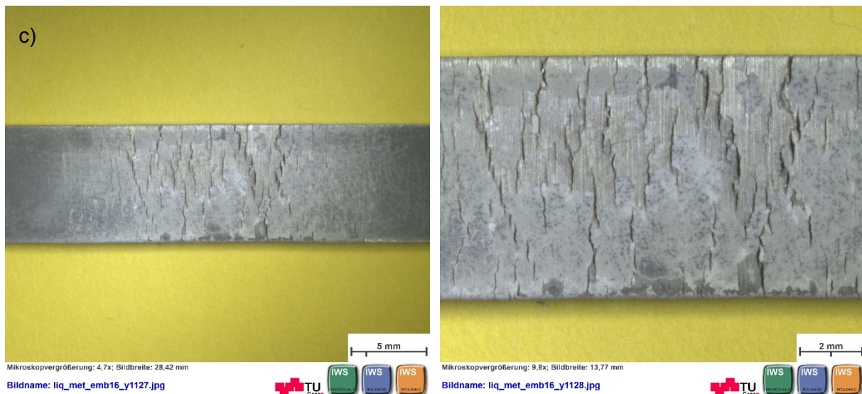
Figure 64: Stereo microscopy images of samples after RSW simulation test procedure at: a) 700°C b) 800°C c) 900°C
