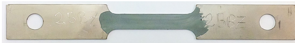
Figure 28: Sample of 301M material with zinc-rich painting
