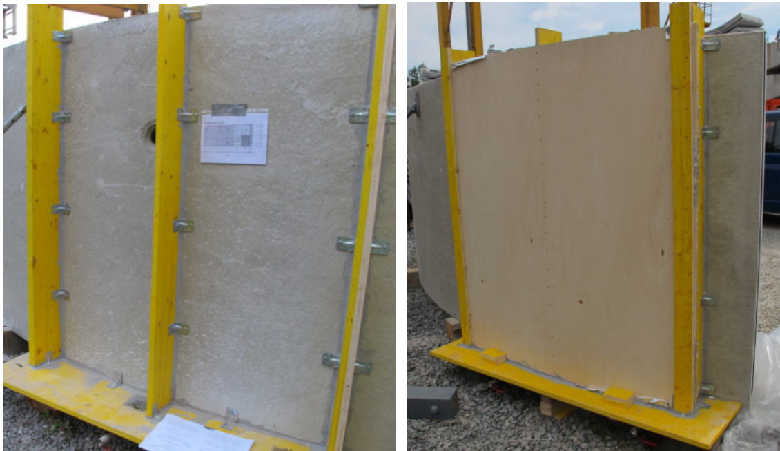
(a) Wooden formwork without “rock” side boundary. (b) Wooden formwork with “rock” side boundary.
