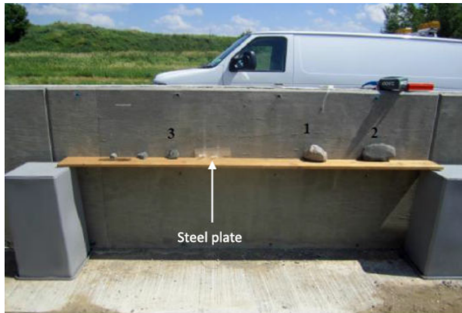
Figure 21: Test setup for the location of rocks behind reinforced concrete wall (taken from Lalagüe et al., 2016).
