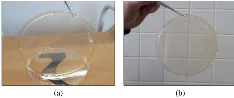
Figure 8. Freestanding film of chitosan (a) and alginate (b) produced using casting method.
