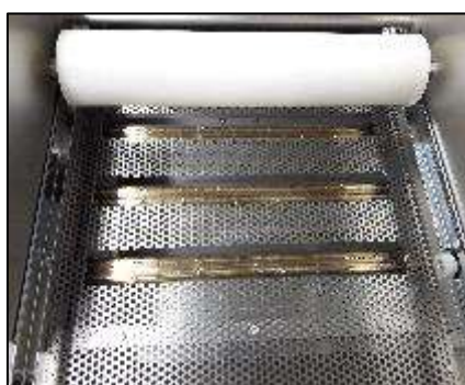
Figure 25. Drying section of the Sumet coater with 3xIR and hot air emitters.
