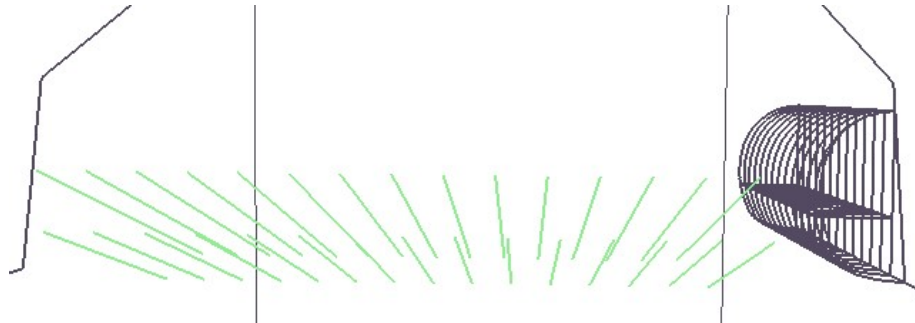
Figure 3.15 Additional anchor row placements
