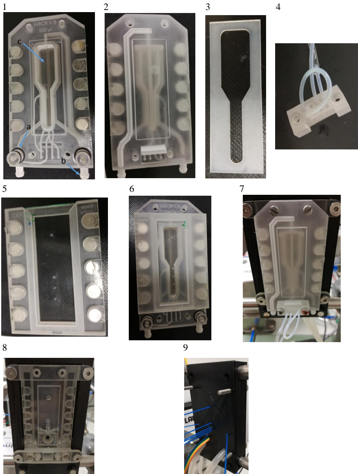
Figure 9: Microbioreactor design: Different parts of the microreactor used for cultivation. 1 microreactor inner view, 1a connection for cooling water, 1b gas in/outlet; 2 microreactor front site; 3 sealing; 4 connector for filling; 5 backside of the reactor composed of a holder and the sensorplate; 6 reactor – back view – including sealing and sensorplate; 7 whole reactor with sensorplate and connector fixed into the docking station providing connection to the cooling system and glass fibres; 8 docking station – front view – stationary part for fixation of the reactor system; 9 docking station – back view – the docking station provides connections to the cooling system and enables positioning of the glass fibres and temperature sensor.
