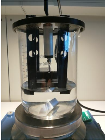
Figure 11: Set-up for stability measurements of the sensor in liquid phase in the incubator (100 % humidity, 5 % CO 2 , 37 °C).
