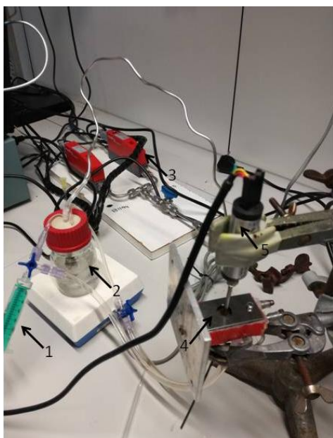
Figure 7: General set-up for measuring response times. In a Schott flask the buffer was saturated with CO 2 (5 or 15 %). The buffer was then manually pumped into a flow-through cell containing the sensor foil. 1 syringe; 2 Schott flask with buffer; 3 MFC; 4 flow through cell; 5 PICCOLO.
