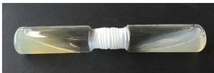
Figure 1 Coincubation setup for GC-MS measurements allowing exchange of volatile organic compounds of two strains without direct contact to each other.
