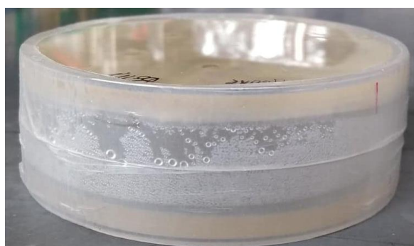
Figure 2 Incubation setup enabling exchange of volatile organic compounds between microorganisms
