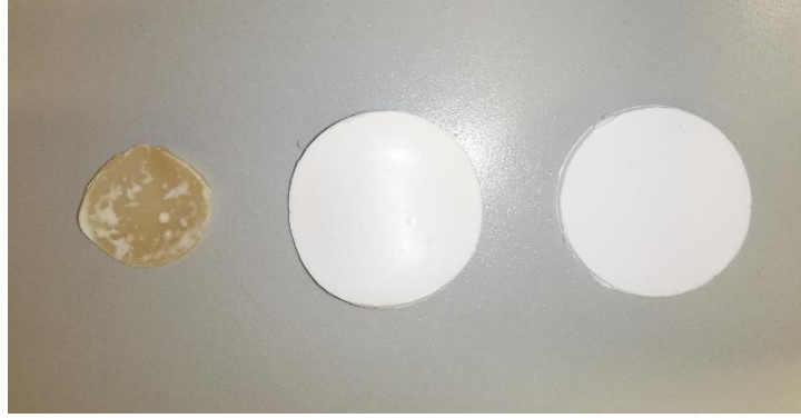
Figure 21. P0 (left) and P40 (middle) after swelling procedure in toluene and sample before swelling procedure in toluene (right).
