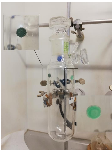
Figure 45. Sensor spots (normal sensor left, trace sensor right) spotted on the experimental flask.
