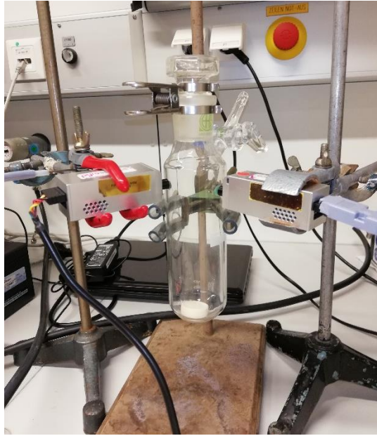
Figure 46. Experimental setup during a simultaneous measurement of normal (left) and trace (right) sensors.
