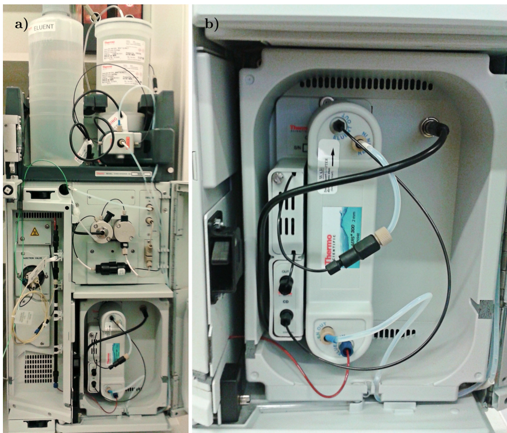
Figure 4.1: a) The Dionex Integrion HPIC system in HPAEC-sCD configuration. b) The correctly plumbed suppressed conductivity detector.
