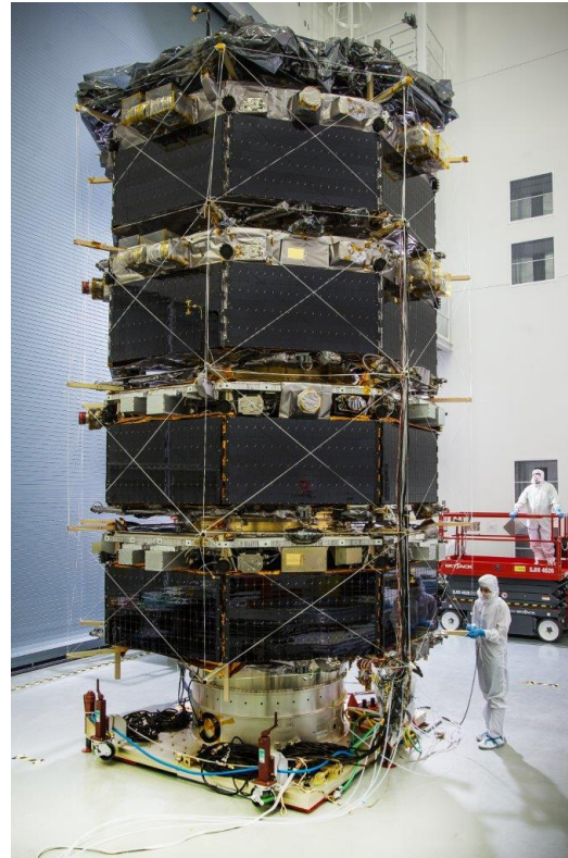
Figure 1–4 MMS Spacecraft Stack (© NASA/Chris Gunn 3 )
