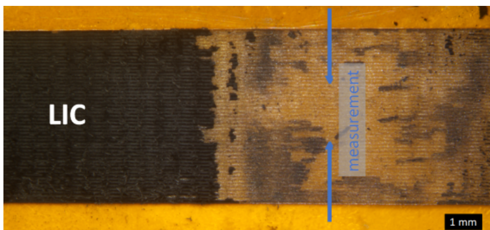
Figure 3.11.: Sample of LIC with a removed part for measuring the thickness of the LIC film produced by laser induced carbonization
