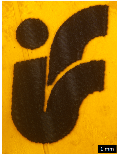
Figure 3.5.: Logo of the Institute of Solid State Physics drawn on top of polyimide with laser induced carbonization
