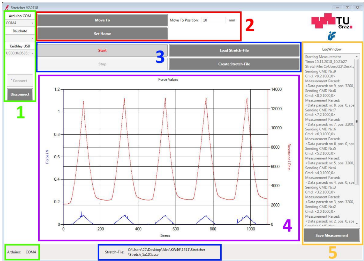
Figure 3.16.: Graphical User Interface: The connectivity panel in green (1), the manual control panel in red (2), the measurement control panel in blue (3), the graph area in violet (4) and the Log-Window in yellow (5)
