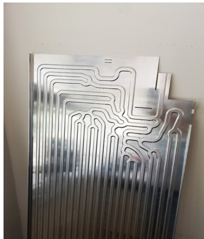
FIGURE 5-10: FORMING VIA ROLL-BONDING
