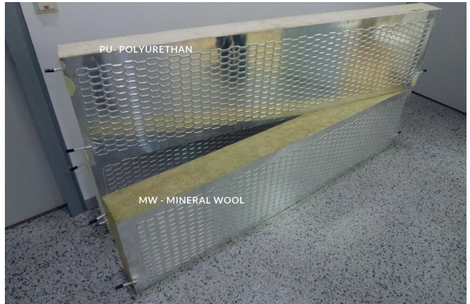
FIGURE 8-1: UNAB FAÇADE PANEL PROTOTYPE
