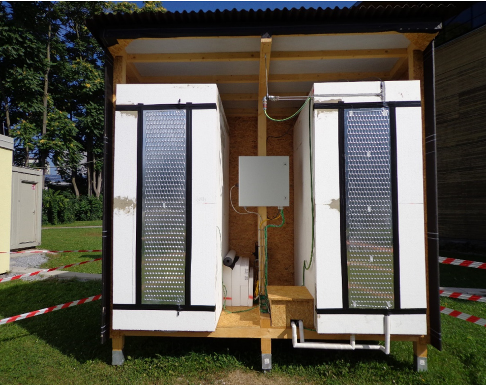
FIGURE 8-4: COMPLETED TEST FACILITY - LEFT, THE NON-ACTIVATED, RIGHT, THE ACTIVATED UNAB FAÇADE PANEL
