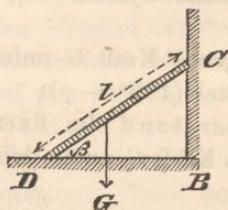
$$180) \left\{ \begin{aligned} C &= \frac{n}{l} \cdot G \cdot \frac{1}{\tan \beta + \mu} \\ D &= G \cdot \left( 1 - \frac{n}{l} \cdot \frac{\mu}{\tan \beta + \mu} \right) \\ K &= G \cdot \left( \frac{n}{l} \cdot \frac{1 + \mu^2}{\tan \beta + \mu} - \mu \right) \end{aligned} \right.$$
