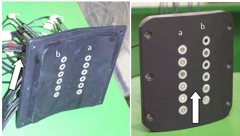
Figure 4-11: Steel plate for the tip microphones (left) and the hub microphones (right)
