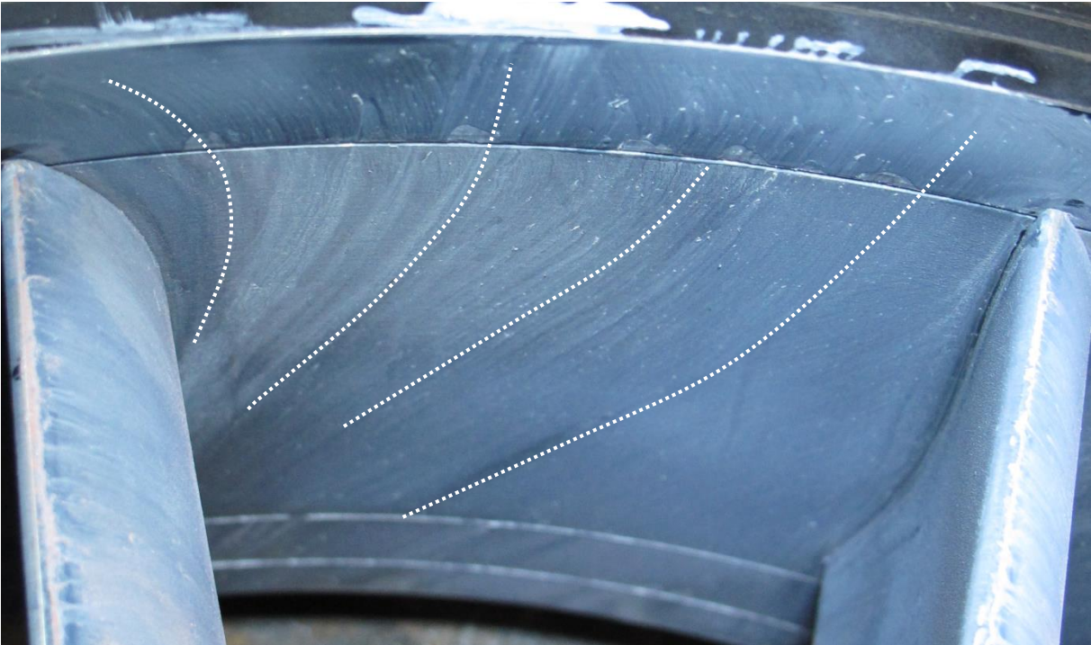
Figure 5-15: Oil flow visualisation “Datum EGV”, operating point ADP; Casing
