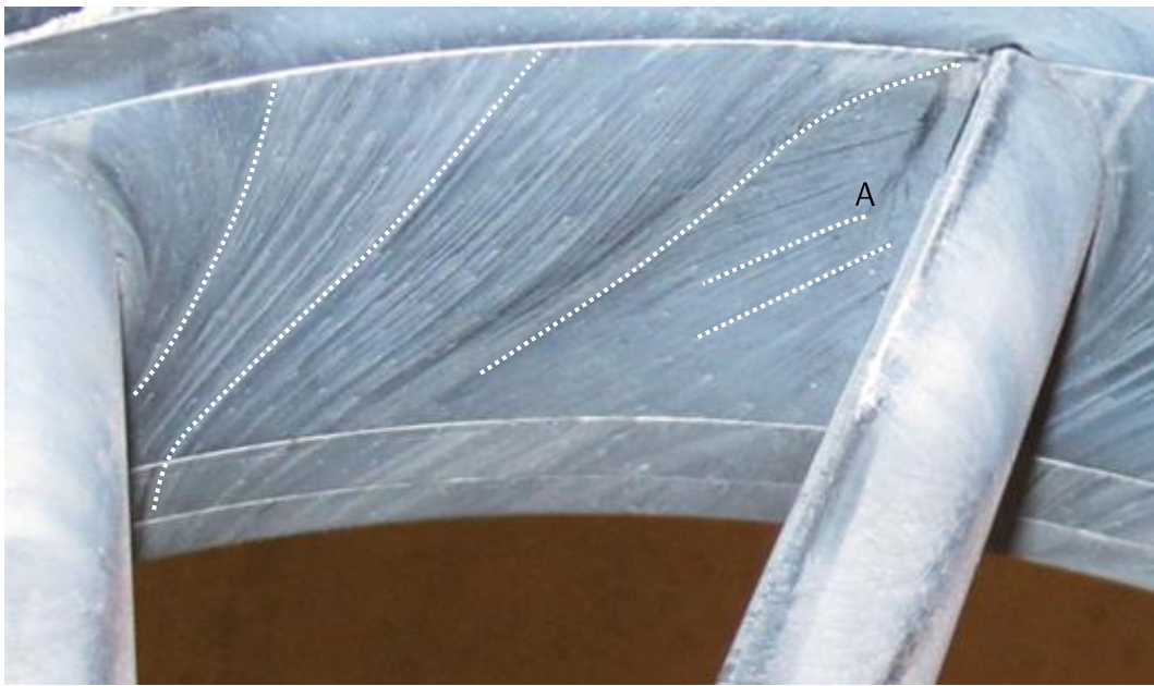
Figure 5-101: Oil Flow visualisation, casing, "Leaned" EGV, operating point Approach
