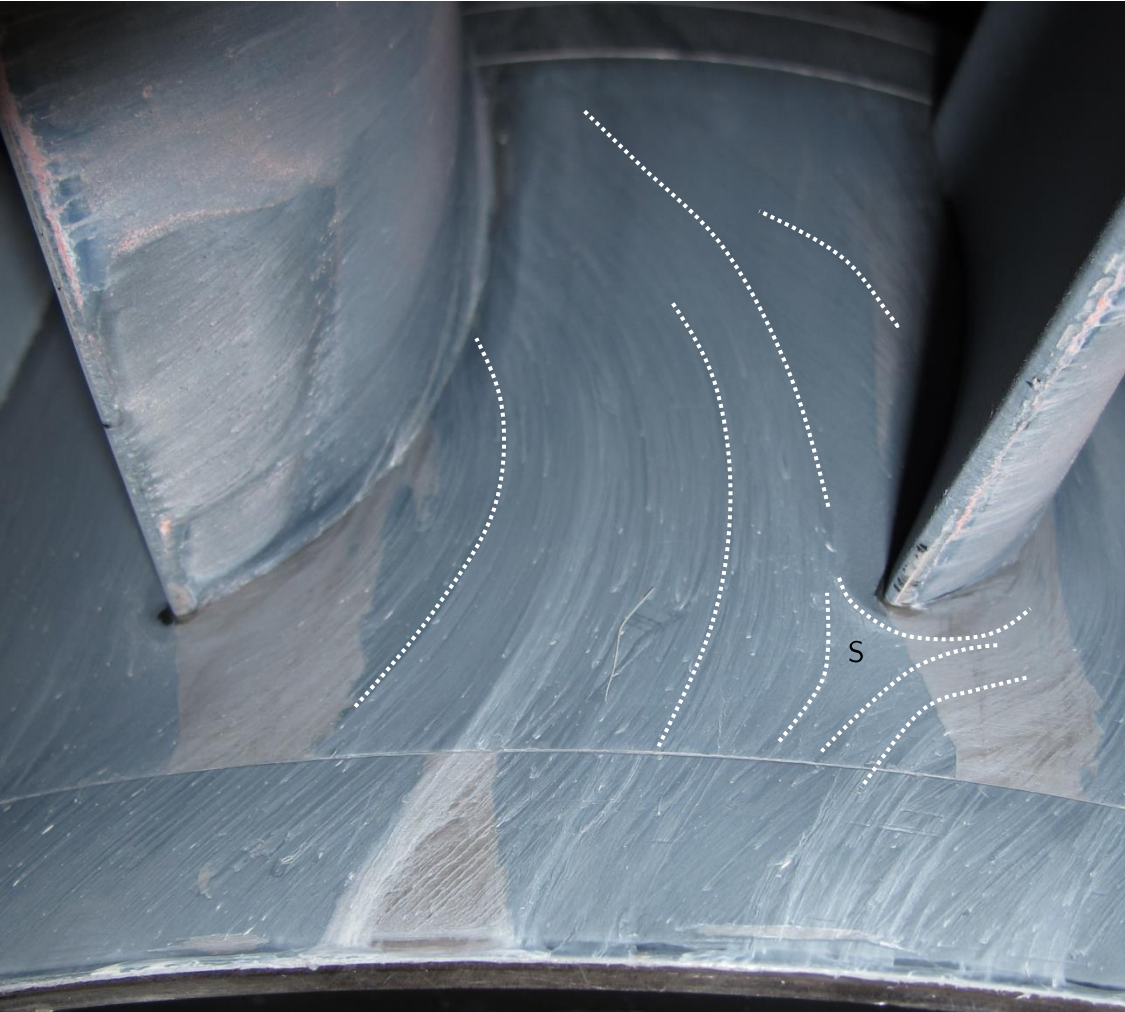
Figure 5-14 Oil flow visualisation “Datum EGV”, operating point ADP; hub
