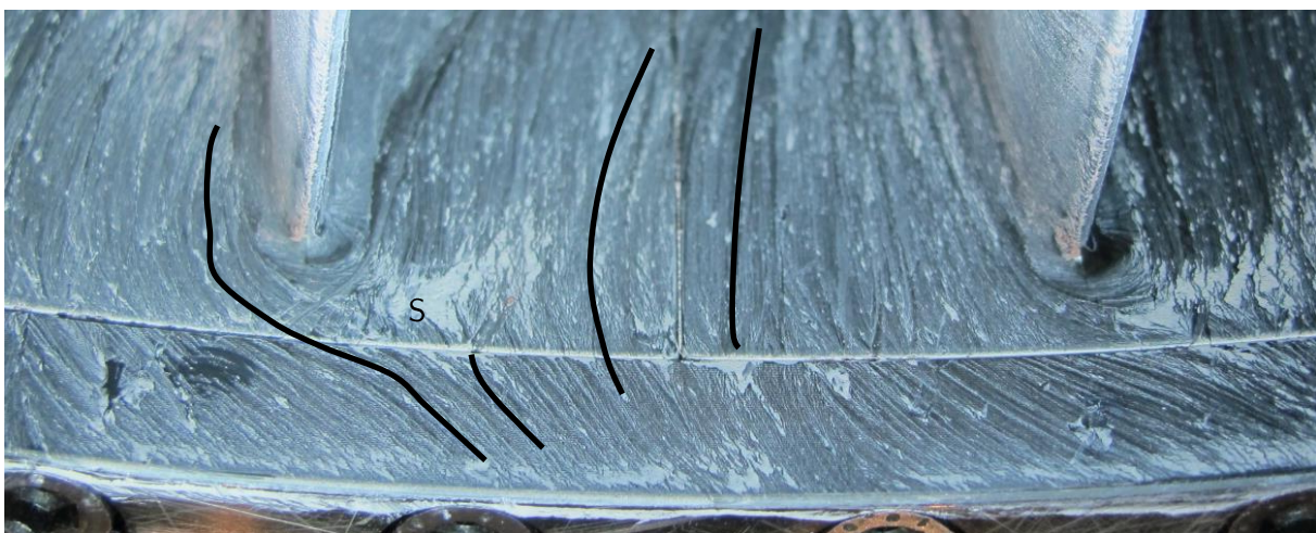
Figure 5-140: Casing Oil Flow visualisation, “High Loading” EGV operating point Approach
