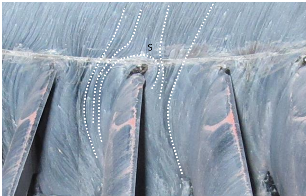
Figure 5-121: Casing Oil Flow visualisation, “Inverse Cut-off” EGV operating point Approach
