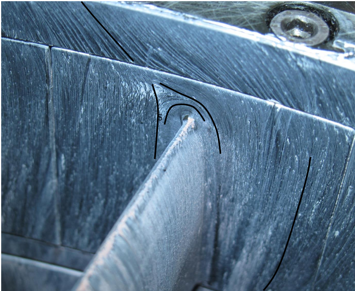
Figure 5-62: Casing oil flow visualisation, "High Loading" EGV, operating point ADP
