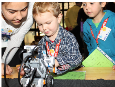
(d) LEGO NXT robot equipped with ultrasonic sensor (topic: intelligent agents (collision avoidance))
