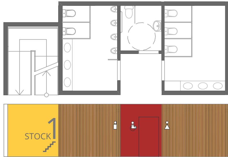
Figure 6.31: Contrasting colors for staircases and toilets help to locate these areas easily
