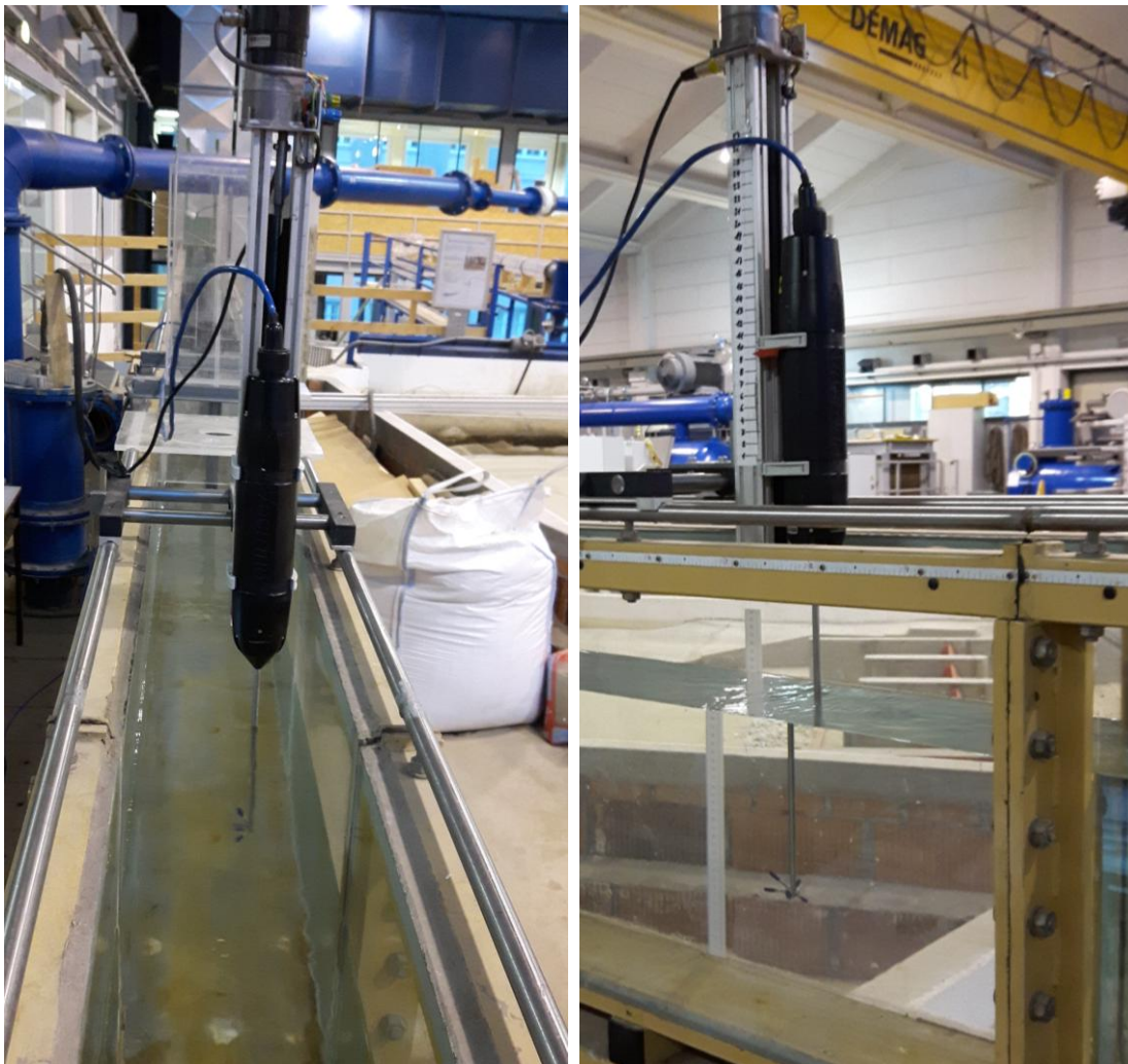
Figures 28 and 29: Installation of the Vectrino+
