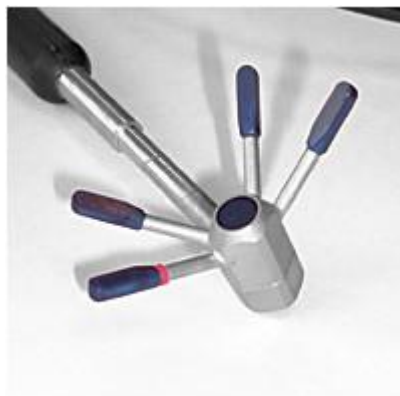
Figure 7: Vectrino side-looking probe [6]
