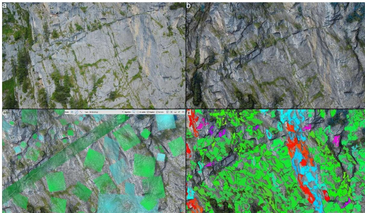
Figure 4-3; (a) original UAV image of a part of the SE-cliff face; (b) respective part of the dense point cloud; (c) manual and semi-automatic plane measurement with CC-Compass; (d) automatic plane extraction with CC-Facets.
