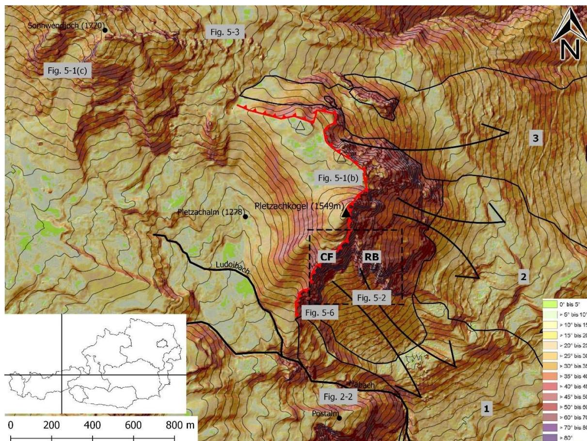
Figure 2-1; Hillshade DEM from 1m Airborne Laser Scan (contour interval 20m) with color coded slope inclination overlay showing the topography of Pletzachkogel and its surroundings.
