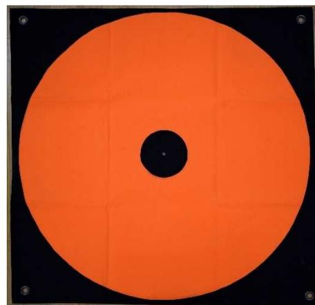
Figure 4-1; GCP specially fabricated for use in alpine terrain
