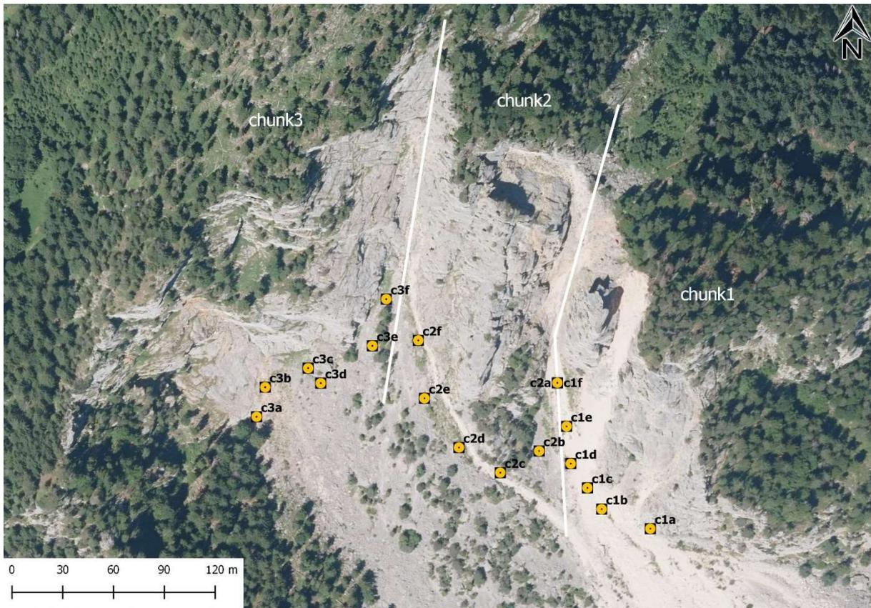
Figure 4-2; Orthophoto of the UAV survey area. The buttress area was divided into chunk 1 & -2, chunk 3 is comprised of the SE- cliff face. The GCPs are marked and labelled corresponding to the table of Appendix 1.
