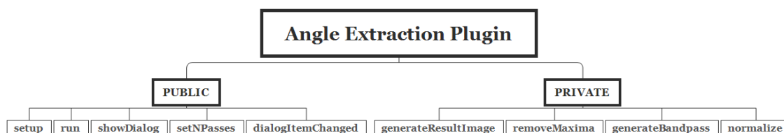
Figure 6.1: An overview of the Java-Methods of the Angle Extraction Plug-in. Private methods are used by the plug-in itself only and public methods can be accessed by external Java code (e.g. ImageJ). This figure does not say anything about the execution order but the accessibility of different methods.
