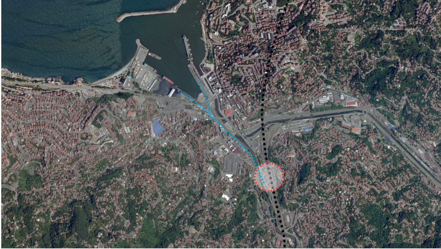
[Figure 123] Location of train station. Black is the train route, blue is the port route for coal transport.
