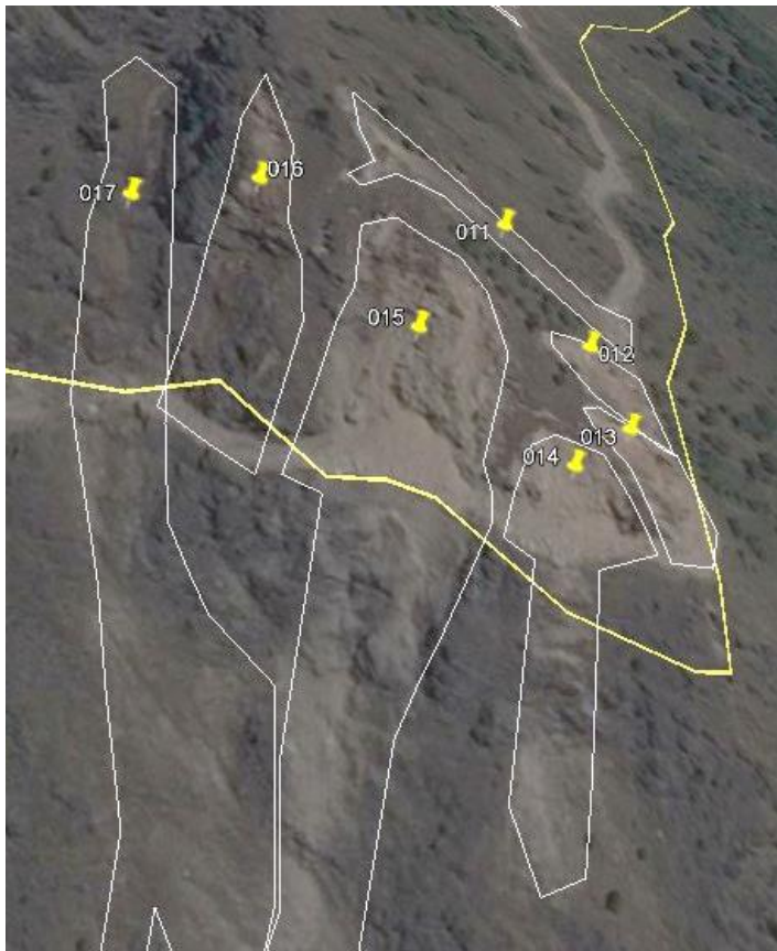
Fig. 10: Google Earth image of landslides affecting a road; Image © 2016 CNES / Astrium.
