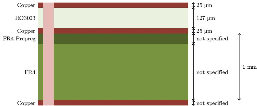
FIGURE 5.12: Stack-up of the mm-wave PCB.
