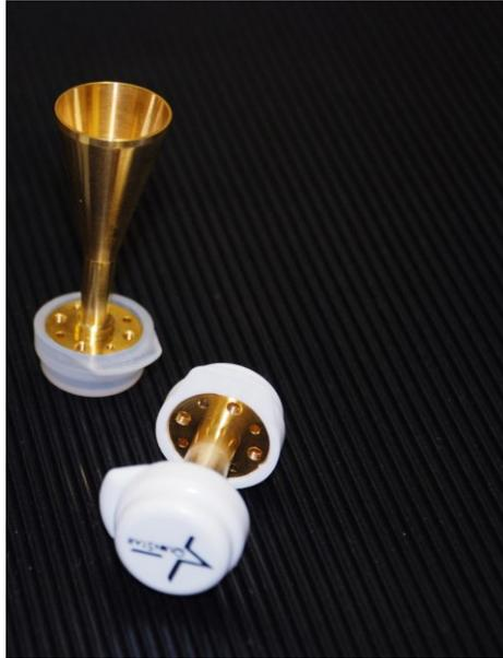
FIGURE 3.2: Picture of the standard gain horn measurement antenna
