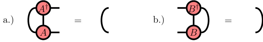
Figure 4: a.) \sum_s (A^s)^\dagger A^s of a left-normalized tensors A yields the identity matrix which we depict as an arc. b.) Similarly BB^\dagger gives the identity matrix if B is right-normalized. It is convention to represent dagged tensors like A^\dagger with the physical index pointing downwards.
