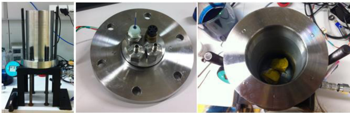
Figure 8.19 Photographic images (© Laura Martínez Vidal) of the pressure chamber consisting of stainless steel tube equipped with metal screws (left), the top fitting with fiber-optic feedthroughs (middle) and the inside of the pressure chamber with a sac (composed of oxygen impermeable aluminum foil) connected to the tube of the manual hand pump (right)
