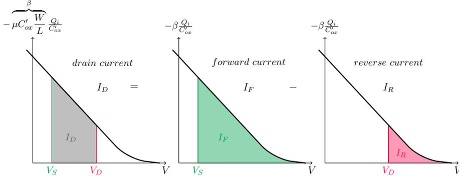
**Figure 6.1:** drain current components,  $V_G = \text{const}$
