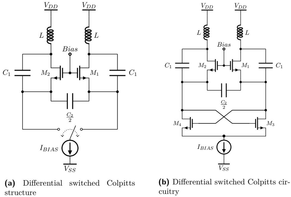
**Figure 3.11:** Advanced Colpitts structures
