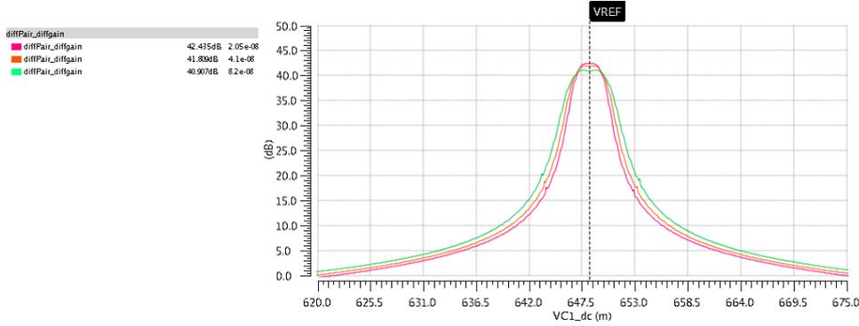
**Figure 8.9:** Simulated transfer for different bias currents
