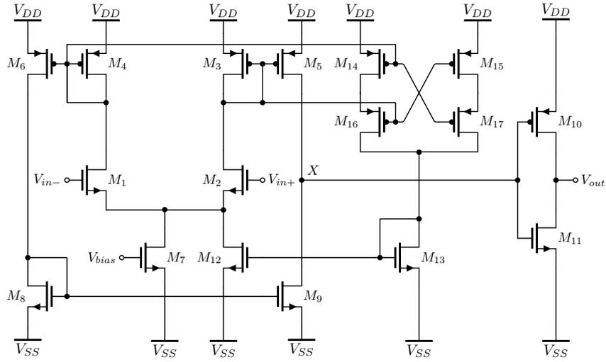
**Figure 5.16:** Modified continuous-time comparator
