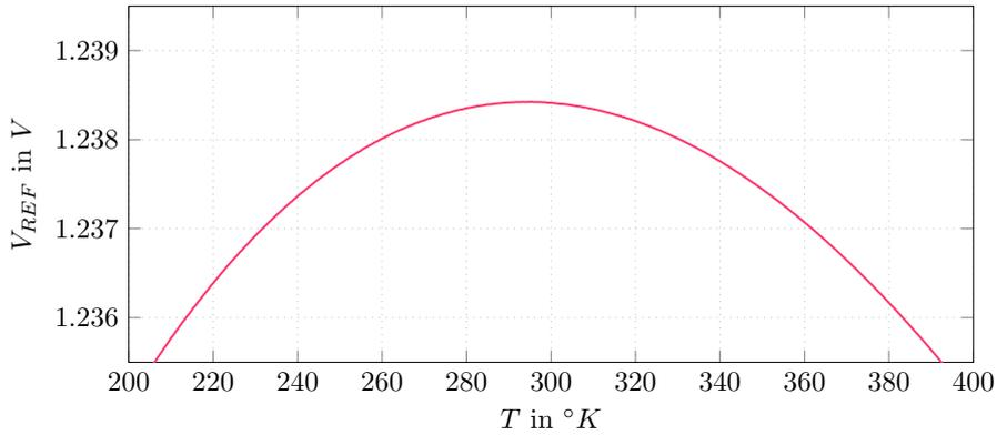
Figure 5.4: Curvature of reference voltage
