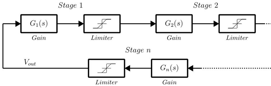
Figure 3.27: Behavioral model ring oscillator
