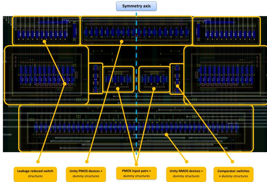
**Figure 10.9:** Layout of the comparator block
