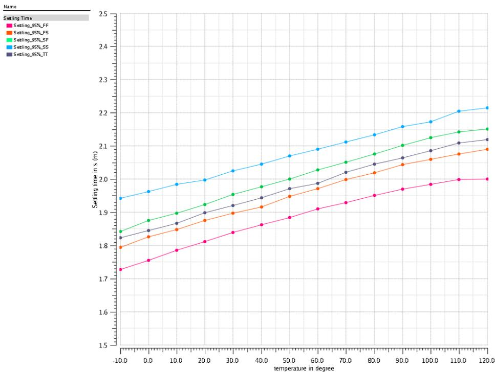
Figure 7.14: Settling time for different corners over temperature
