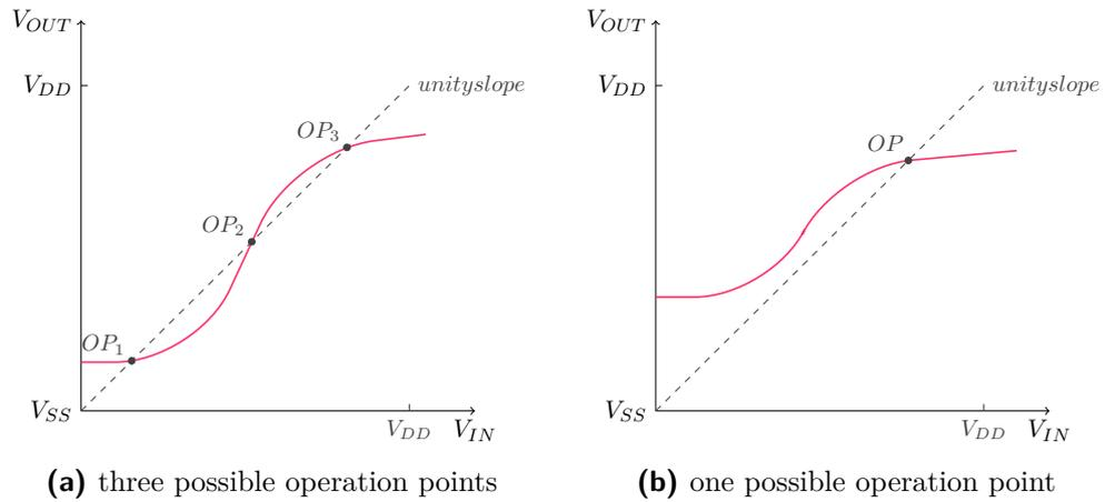
**Figure 7.8:** Broken loop transfer characteristics
