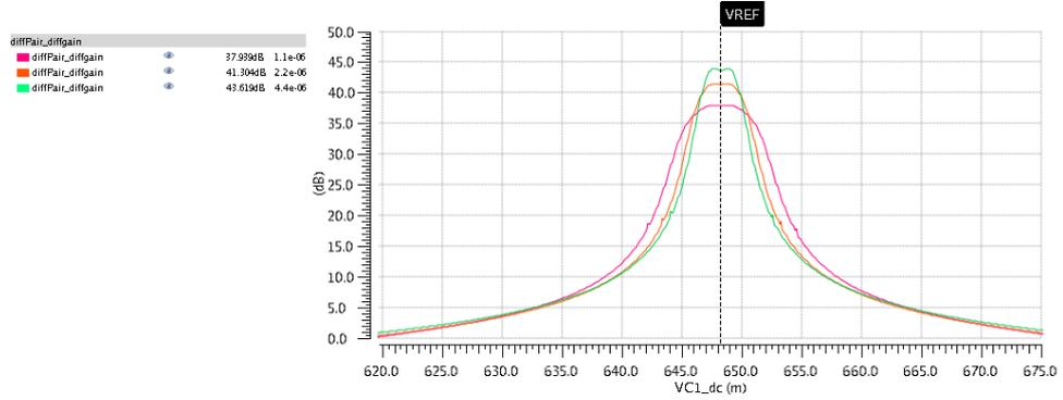
**Figure 8.10:** Simulated transfer for different lengths
