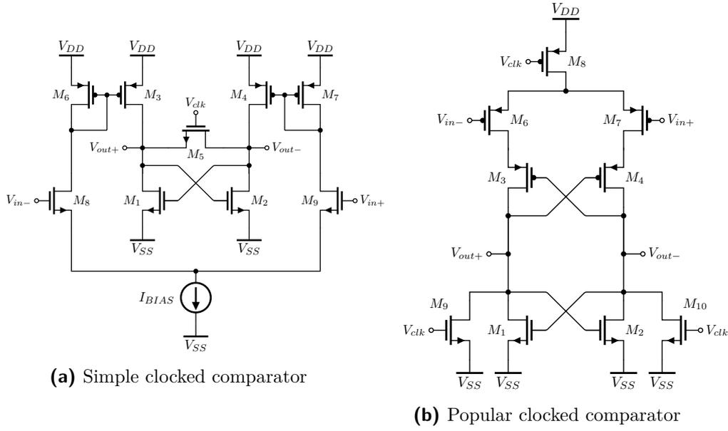
**Figure 5.9:** Common clocked comparator circuits
