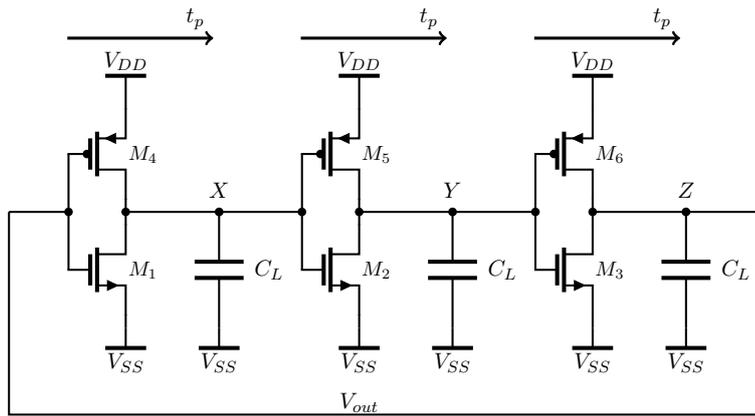
**Figure 3.30:** Inverter based ring oscillator
