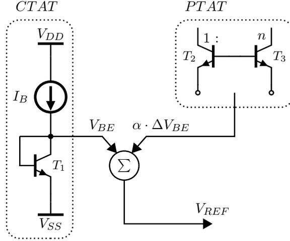
**Figure 5.2:** Principle of a bandgap reference
