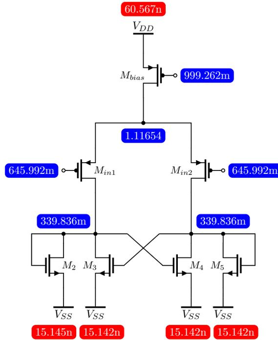
Figure 8.11: Voltages and currents balanced pre-amplifier
