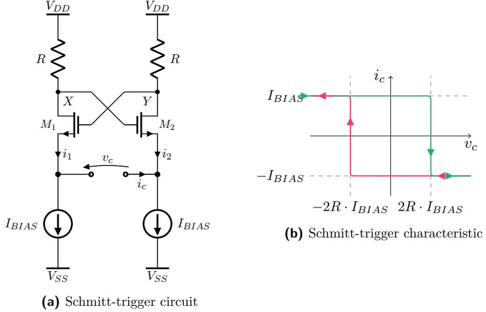
**Figure 3.14:** Schmitt-trigger differential RC oscillator
