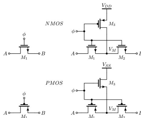
**Figure 9.4:** Simple and reduced leakage switch
