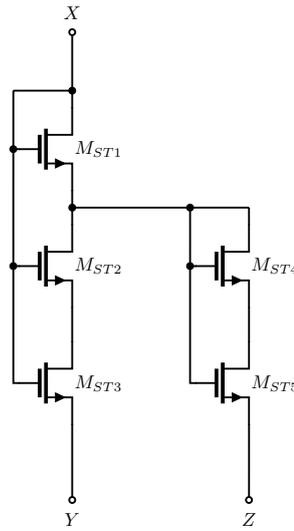
**Figure 7.11:** Start-up circuit of reference generator
