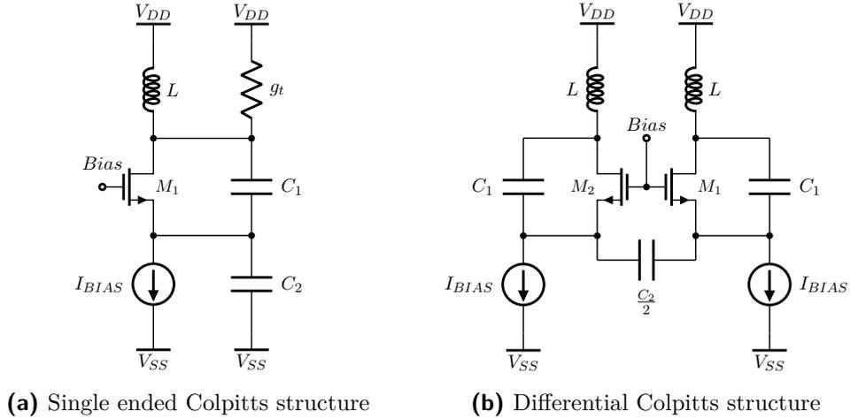
**Figure 3.10:** Basic Colpitts structures
