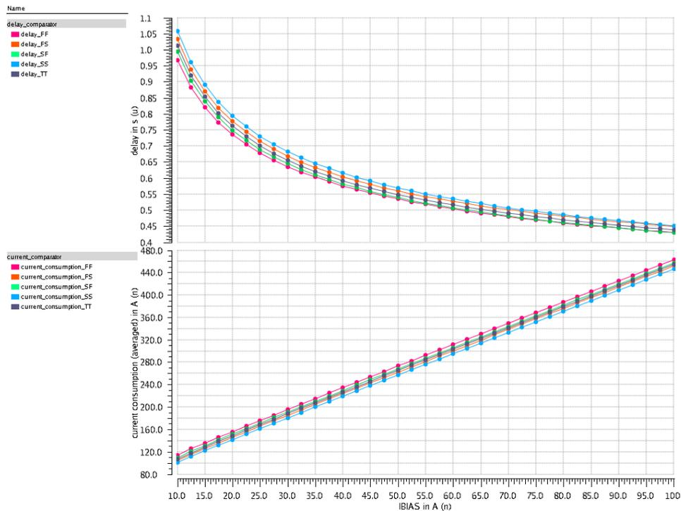
Figure 8.13: Delay and current consumption vs bias current
