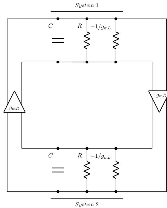
Figure 3.22: Linear model two integrator oscillator
