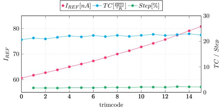
Figure 9.9: Simulated trim characteristics
