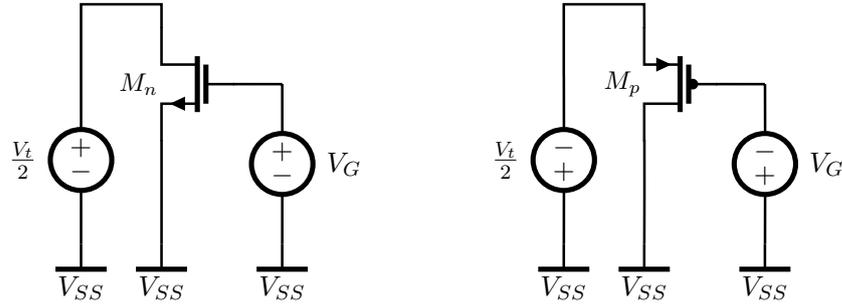
**Figure 6.3:** Principle of extracting  $I_{SQ}$  and  $V_{T0}$ .  $V_B = V_{SS}$ .
