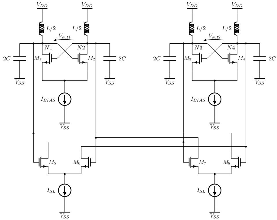
**Figure 3.7:** LC based coupled oscillator
