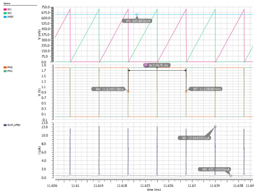
**Figure 9.2:** Transient simulation of the low-power oscillator
