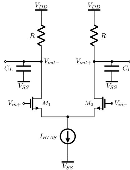
Figure 3.32: Basic differential delay cell
