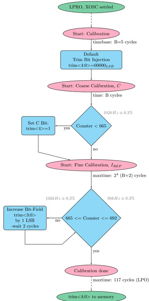
Figure 10.6: Calibration flowchart
