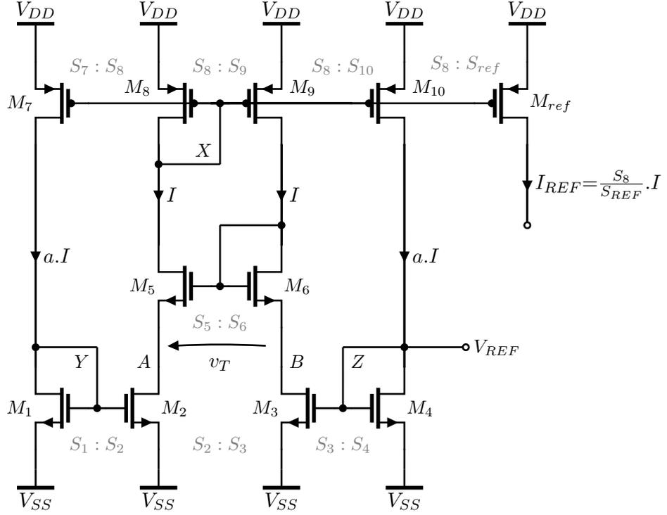
**Figure 7.1:** Principle of the proposed reference circuit
