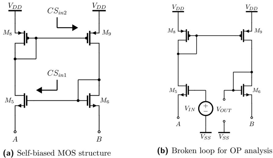
**Figure 7.7:** Reference generator operation point analysis
