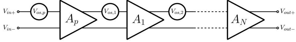
**Figure 5.10:** Multi stage comparator
