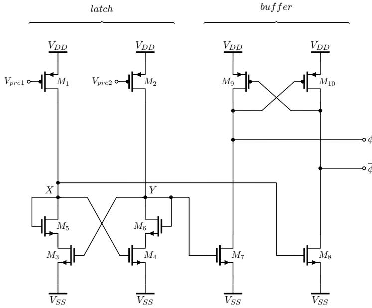
**Figure 8.7:** Latch and buffer stage of comparator
