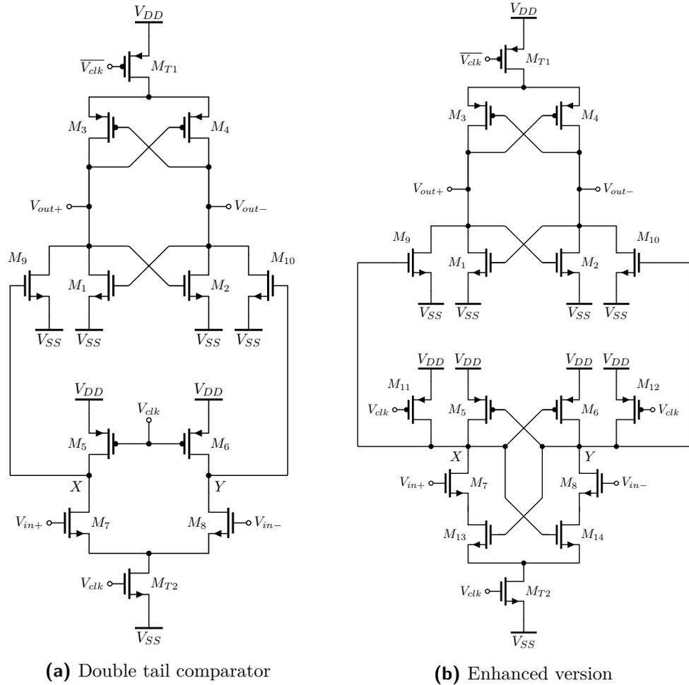
**Figure 5.11:** Double-tail comparator circuits
