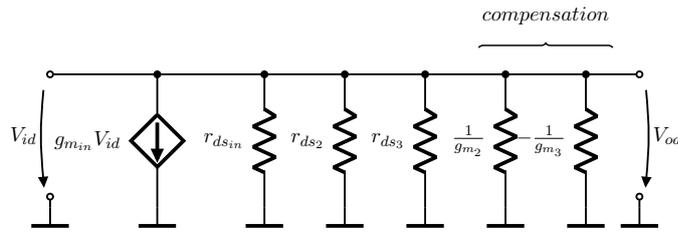
Figure 8.3: Differential-mode small signal analysis
