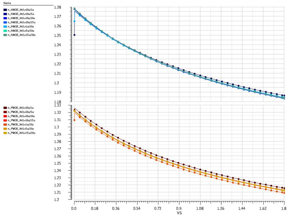
Figure 6.8: Extraction of  $n$  over  $V_S$  for different sizes
