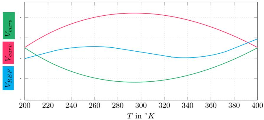
Figure 5.5: Compensation of bandgap curvature
