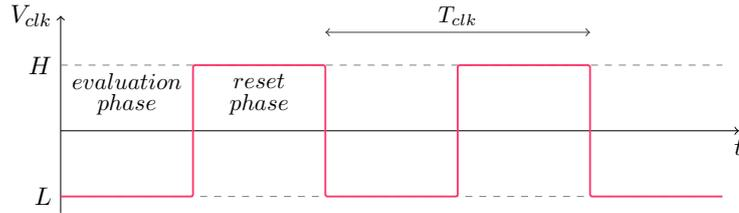
Figure 5.8: Clock signal comparator
