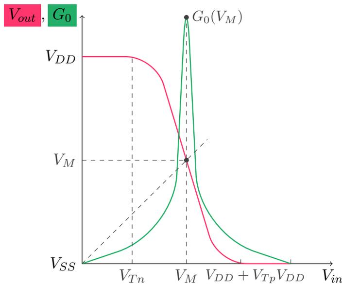
**Figure 3.31:** Inverter characteristics
