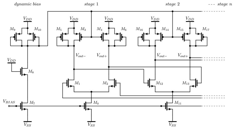
**Figure 3.34:** Differential ring oscillator based on Maneatis delay cells
