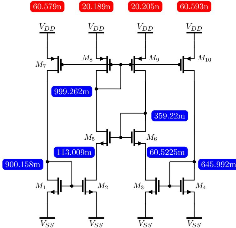
Figure 7.2: BSIM: DC operating point of reference generator
