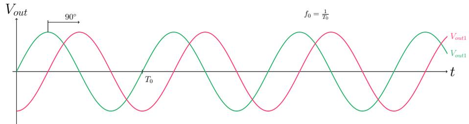
**Figure 3.8:** Output waveforms coupled LC oscillator
