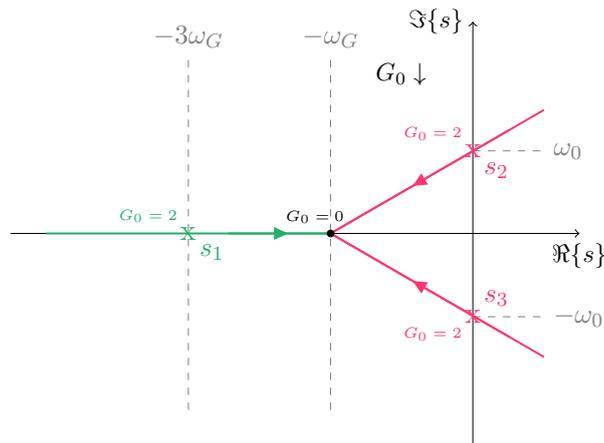
**Figure 3.29:** Pole movement - 3 stage ring oscillator
