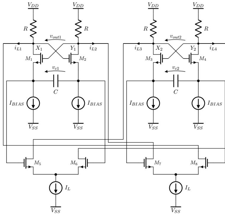
**Figure 3.18:** Coupled RC oscillator circuit
