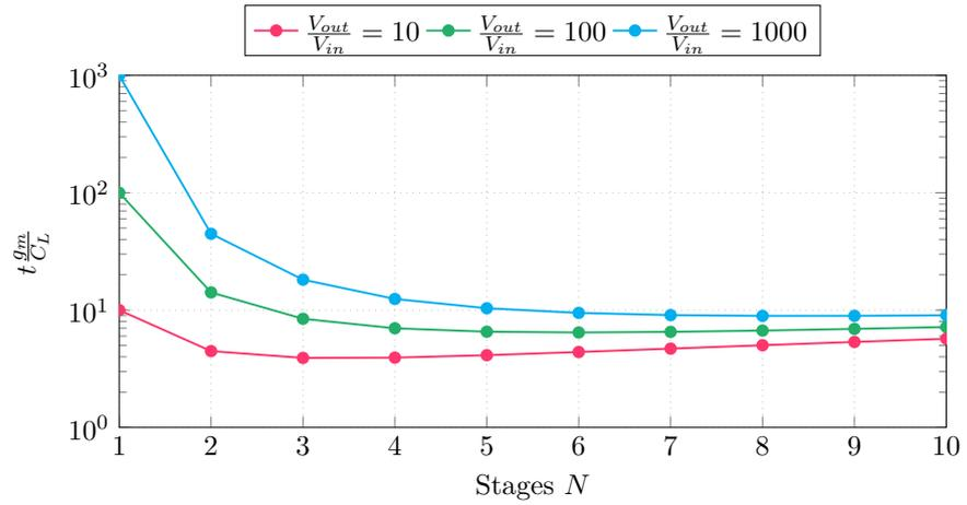
**Figure 5.13:** Number of stages vs. normalized delay
