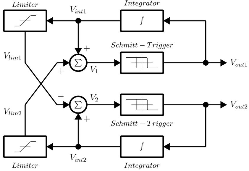
**Figure 3.16:** Behavioural model of coupled RC oscillator
