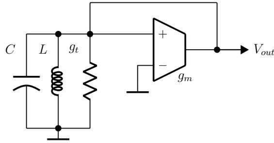
**Figure 3.3:** Structure of a LC based oscillator
