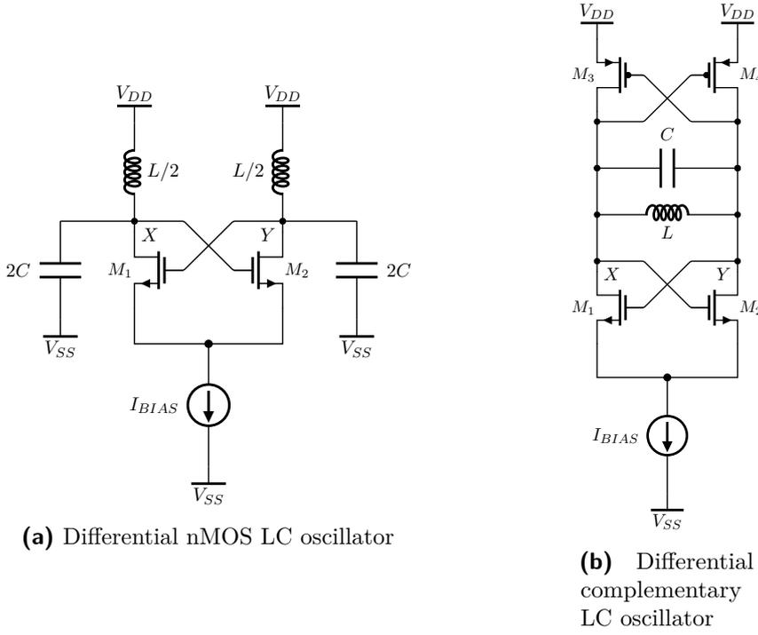
**Figure 3.6:** Differential LC circuits
