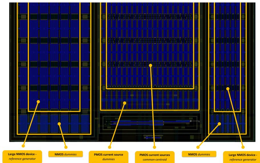
**Figure 10.10:** Layout view of matched devices
