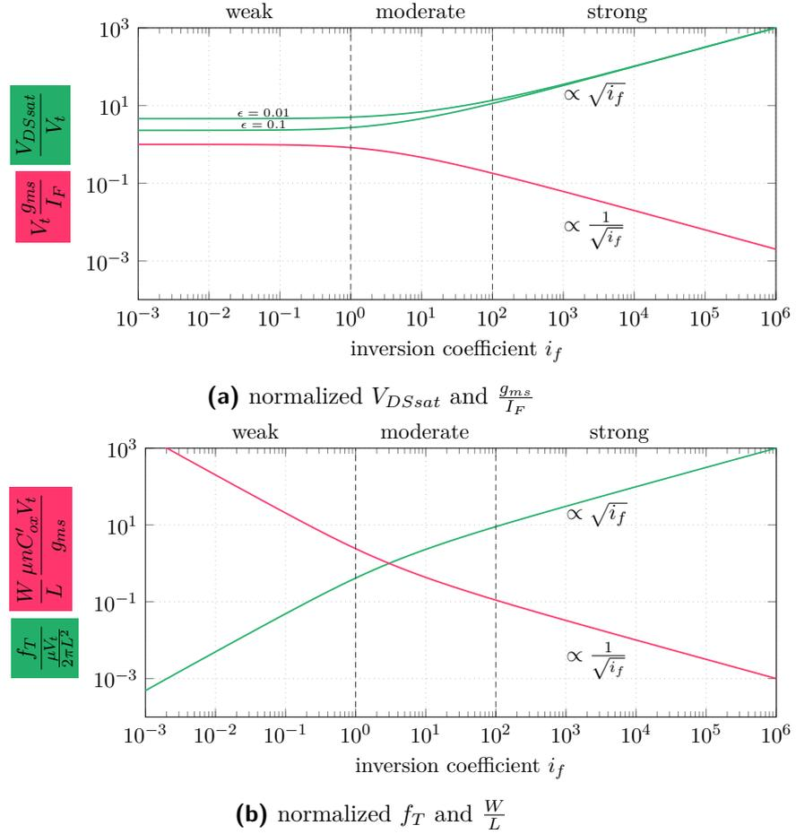
**Figure 6.2:** inversion coefficient as design variable
