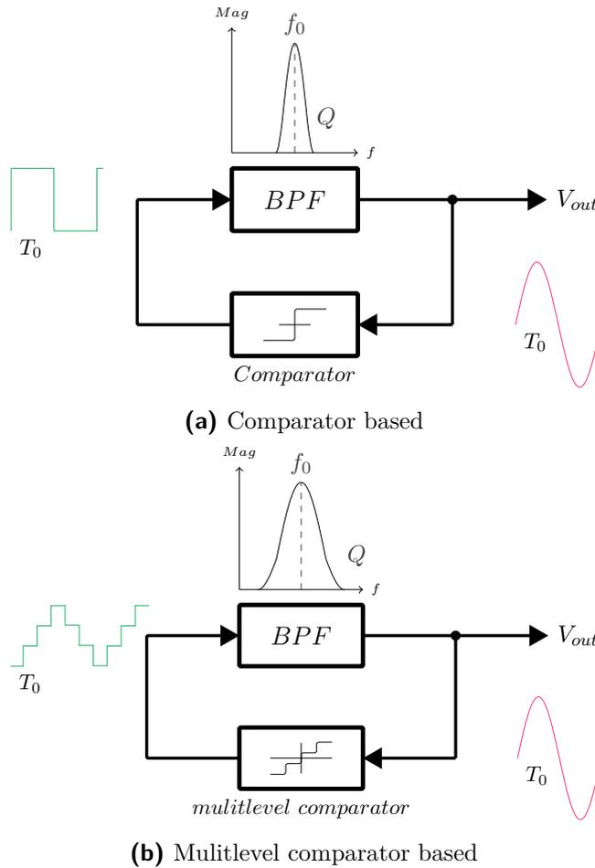
Figure 3.40: Digital feedback oscillators
