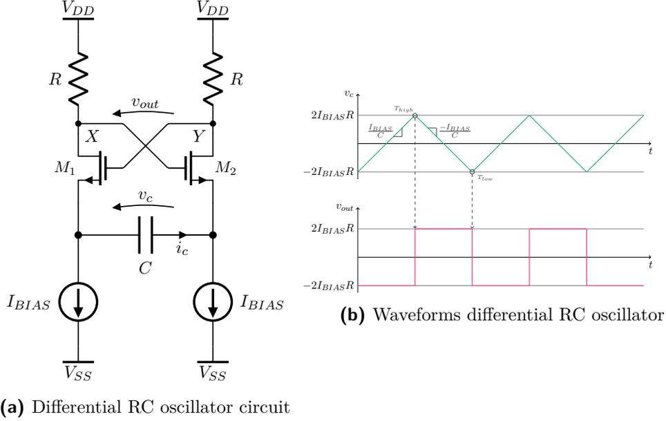
Figure 3.13: Differential RC oscillator
