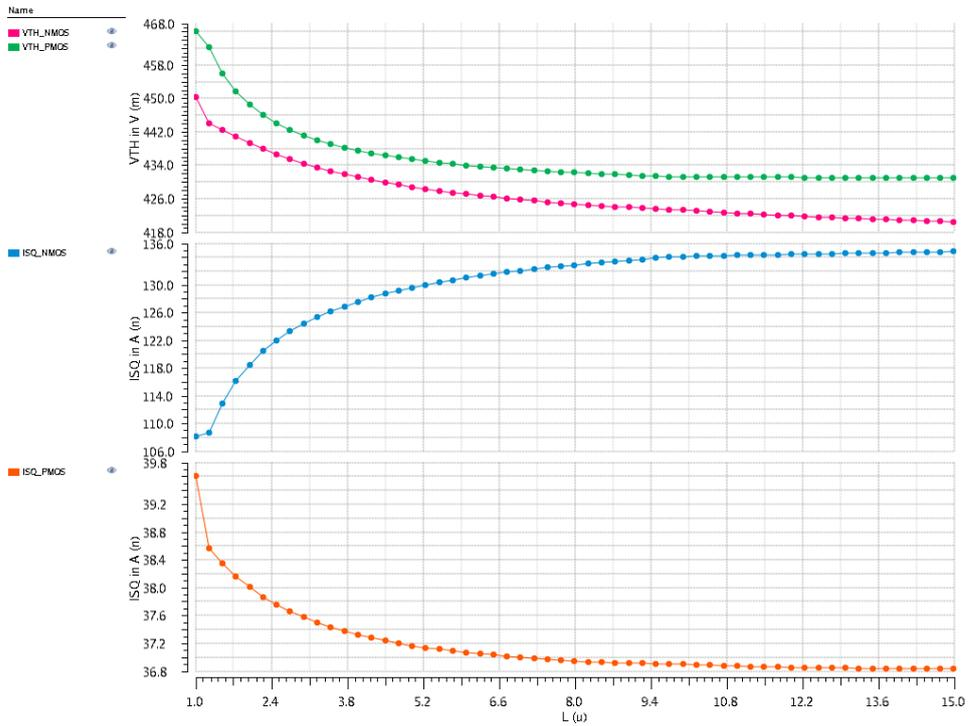
Figure 6.6: Extraction of  $I_{S\Box}$  and  $V_{T0}$  over  $L$ .  $W=10\mu m$ .
