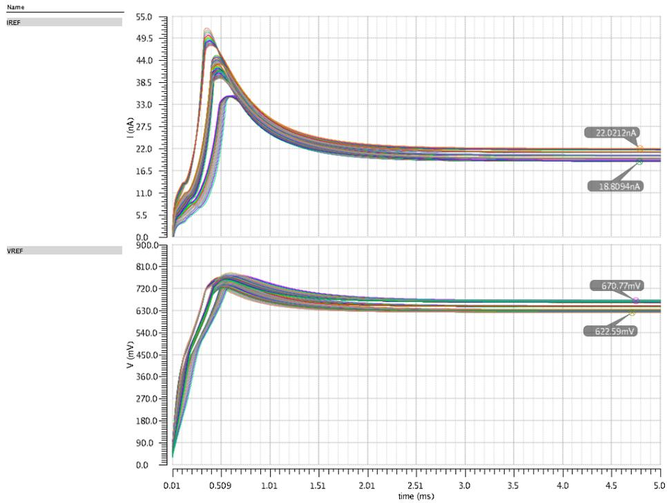
Figure 7.13: Transient waveform of settling over corners and temperature
