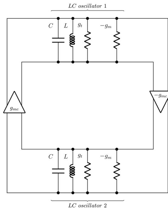
Figure 3.9: Linear model coupled LC oscillator
