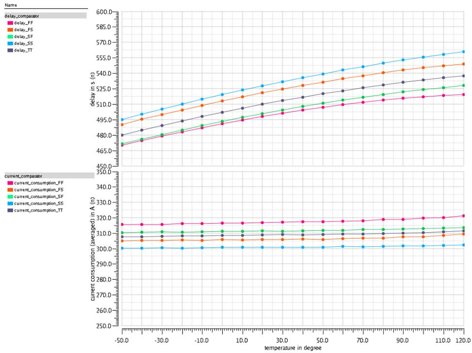
Figure 8.14: Delay and current consumption vs temperature
