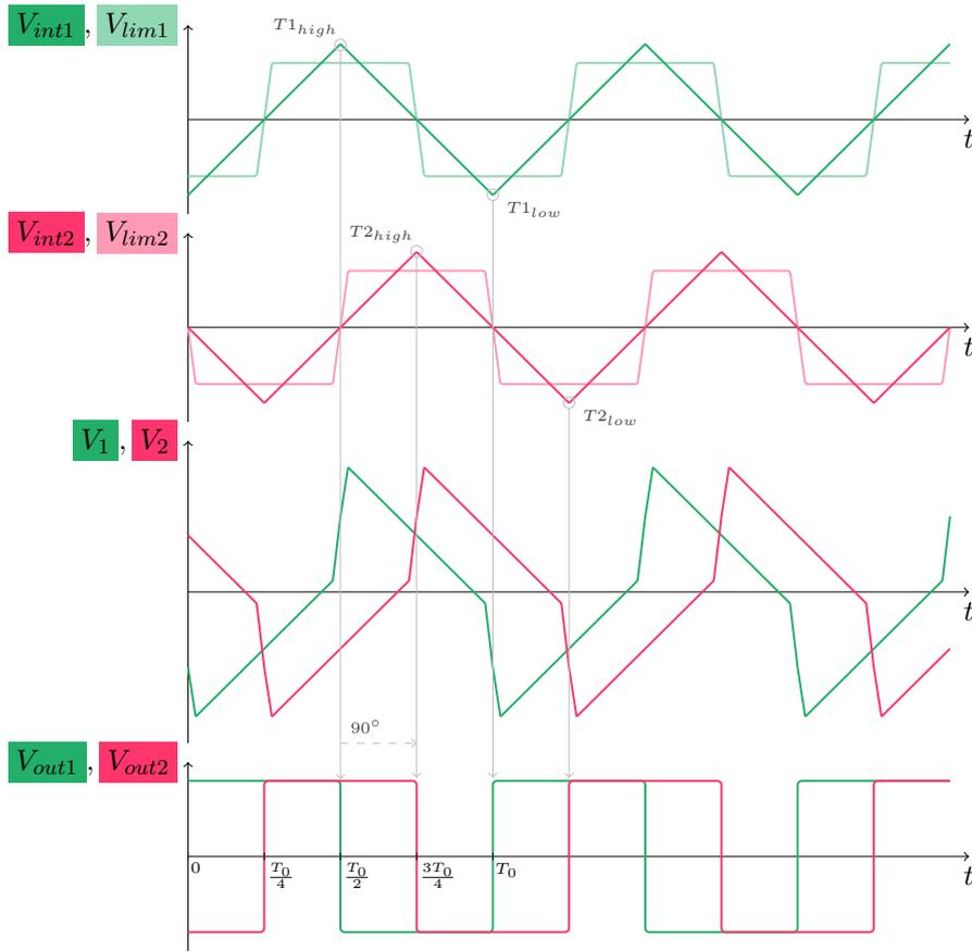
**Figure 3.17:** Waveforms of coupled RC oscillator model
