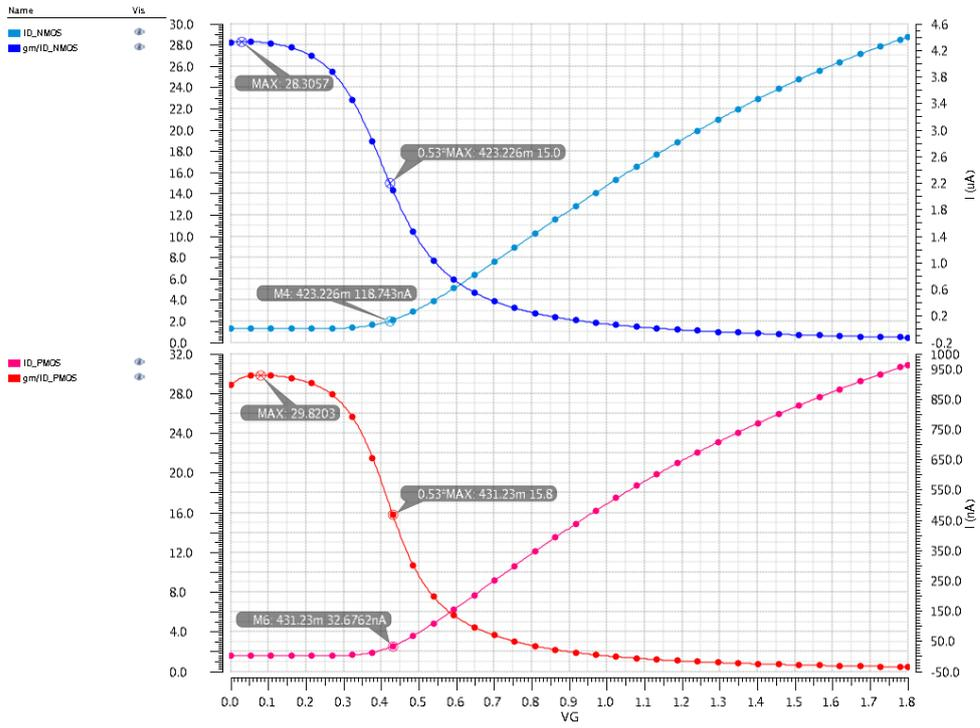
Figure 6.5: Extraction of  $I_{S\Box}$  and  $V_{T0}$  for  $L=W=10\mu m$
