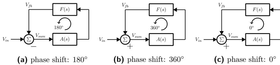
**Figure 2.2:** Various views of oscillator feedback
