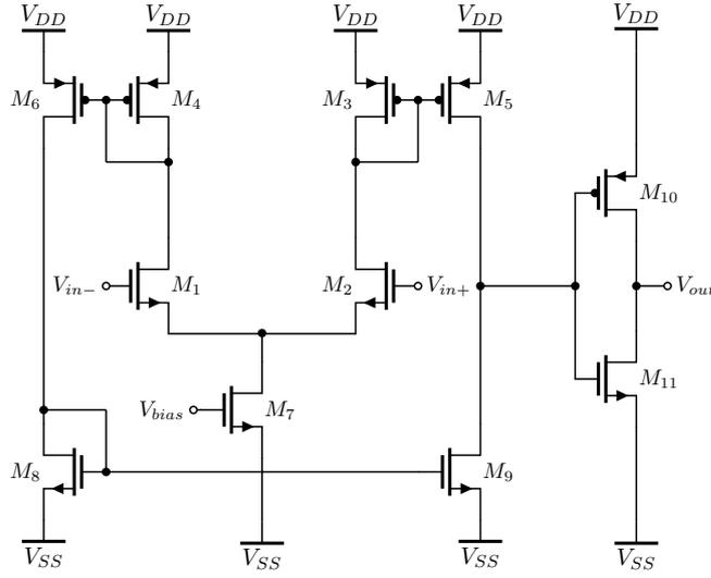
**Figure 5.15:** Simple continuous-time comparator
