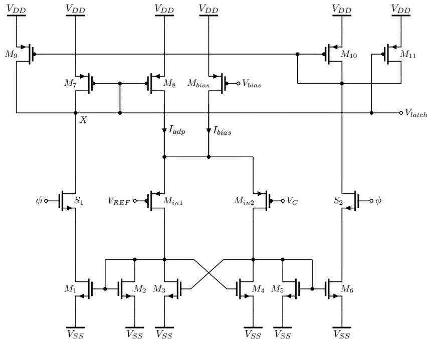
Figure 8.2: Input stage of comparator
