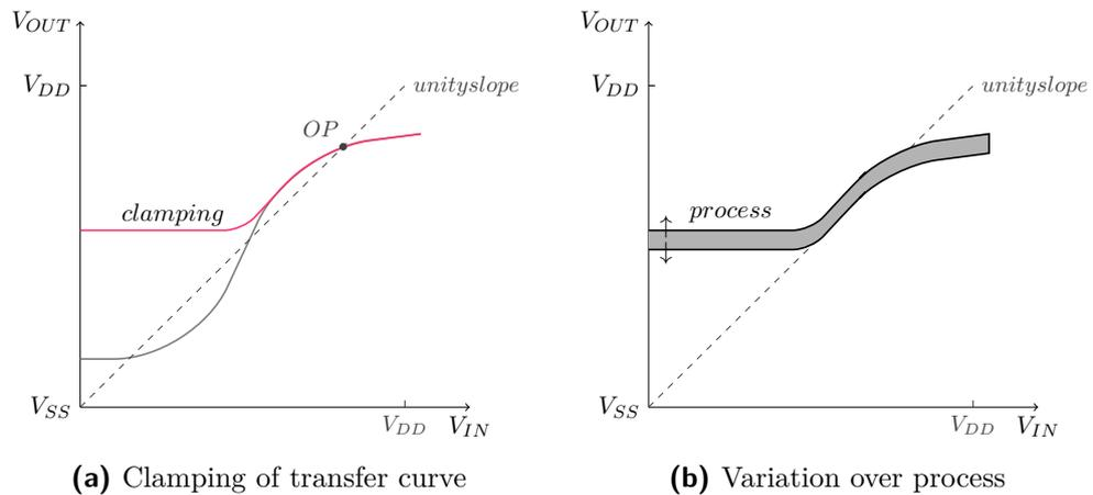
**Figure 7.9:** Transfer characteristics after adding start-up
