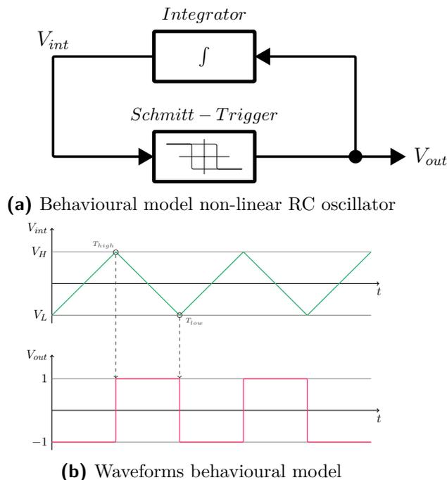
**Figure 3.12:** Non-linear RC oscillator model
