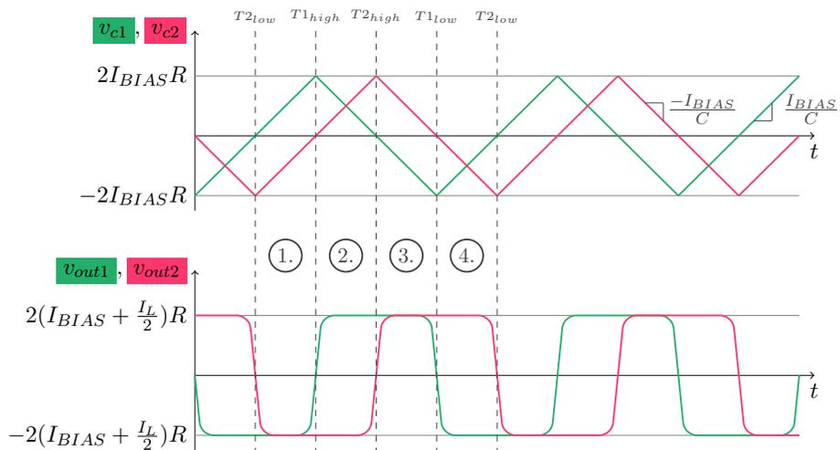
**Figure 3.19:** Waveforms of coupled RC oscillator circuit
