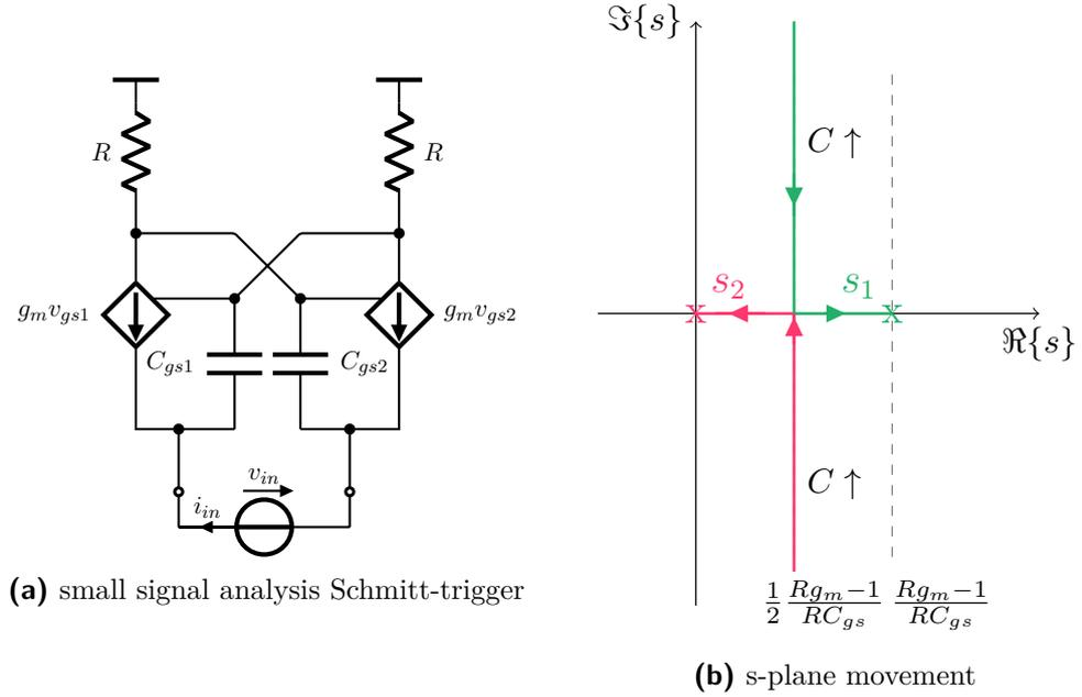
**Figure 3.15:** Schmitt trigger - analysis
