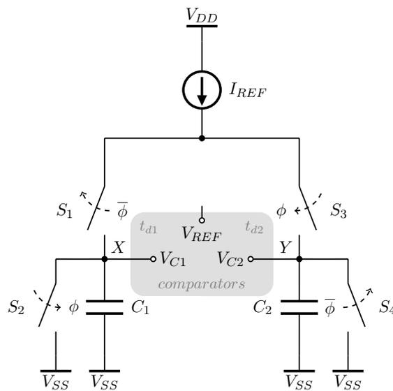
**Figure 9.1:** Time-constant of dual-phase oscillator
