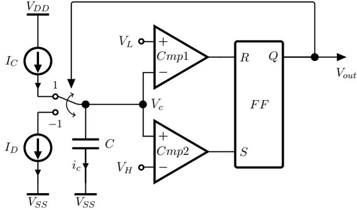
**Figure 3.23:** Double comparator circuit
