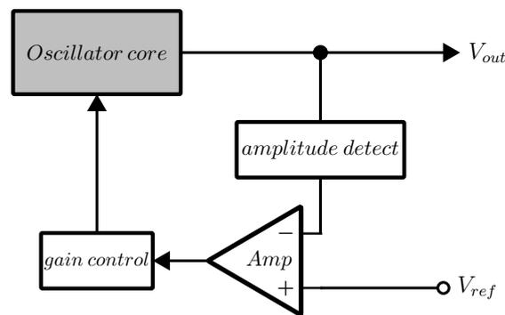
**Figure 2.4:** Amplitude control loop
