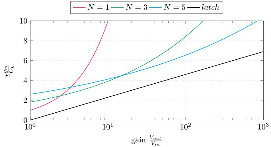
**Figure 5.14:** Gain vs. normalized delay
