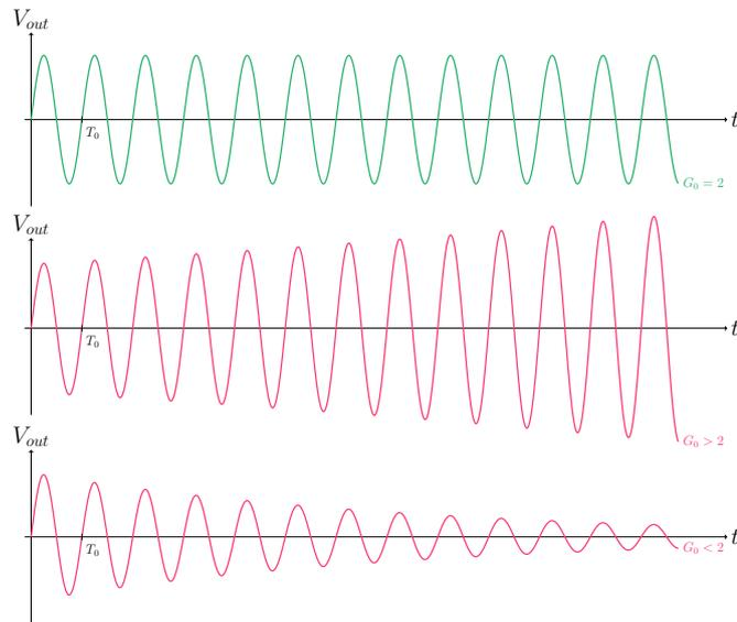
**Figure 3.28:** Signals behaviour - 3 stage ring oscillator
