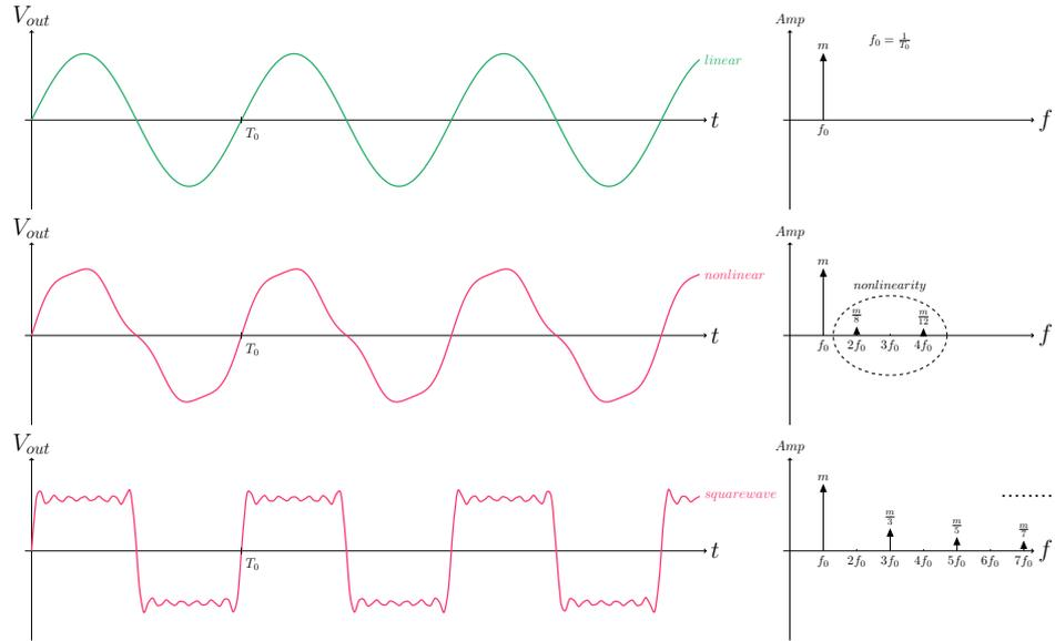
**Figure 3.2:** Output waveforms - linear and non-linear system
