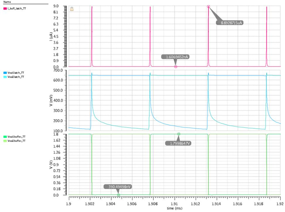
**Figure 8.8:** Current and voltage waveforms of the latch and buffer stage
