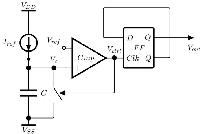
Figure 3.25: Single comparator circuit
