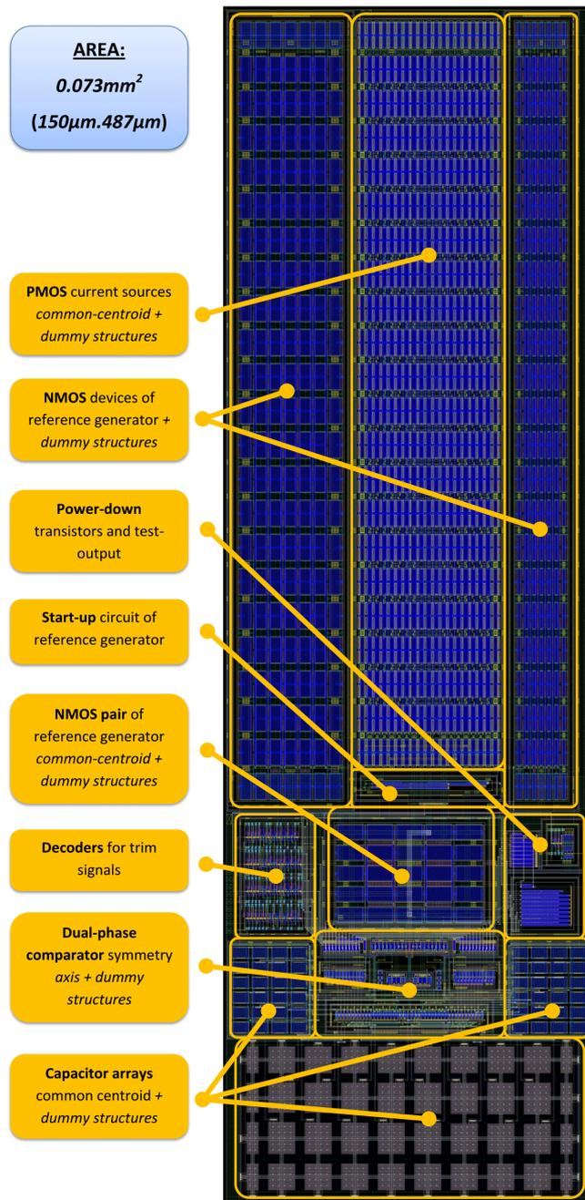
**Figure 10.8:** Layout of the Low-Power Oscillator
