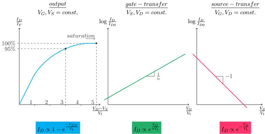
Figure 6.9: Forward characteristics
