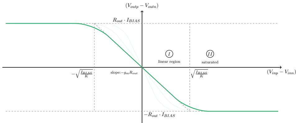
Figure 3.1: Large signal - differential pair
