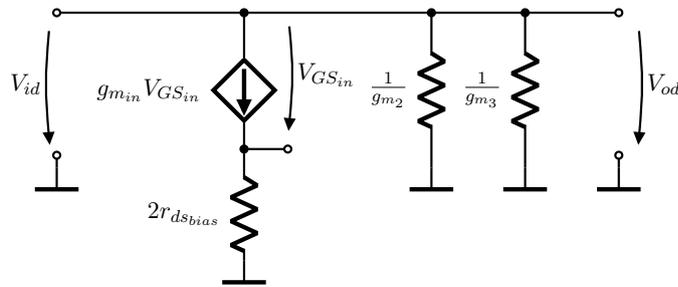
Figure 8.4: Common-mode small signal analysis
