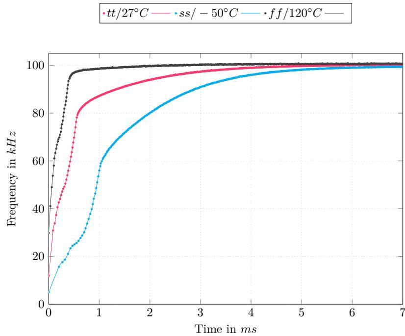
**Figure 10.1:** Settling time over corners
