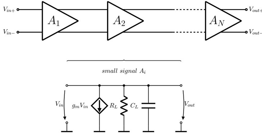
**Figure 5.12:** Small signal behaviour of comparator
