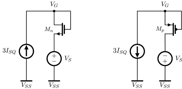
**Figure 6.4:** Principle of extracting  $n$ .  $V_B = V_{SS}$ .
