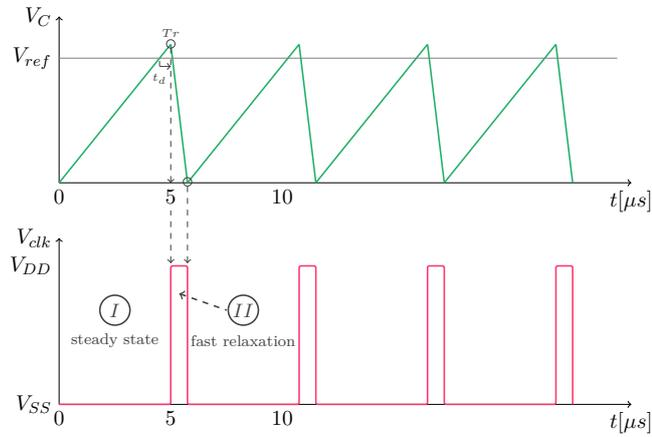
**Figure 2.3:** Waveform example of an integrated relaxation oscillator
