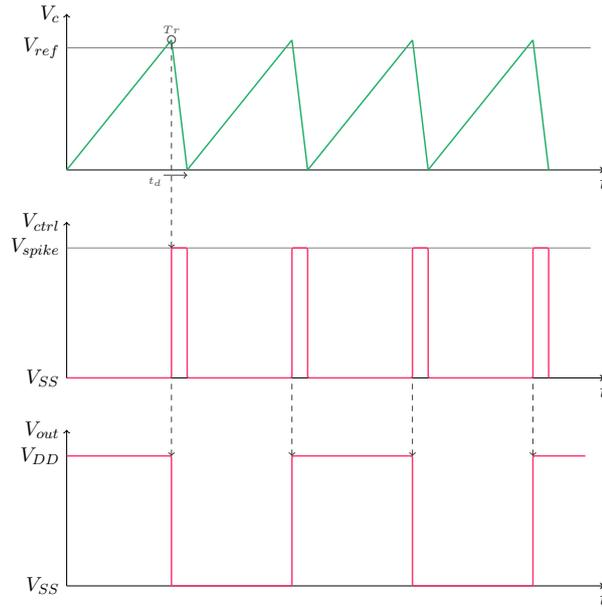
**Figure 3.26:** Single comparator RO - waveforms
