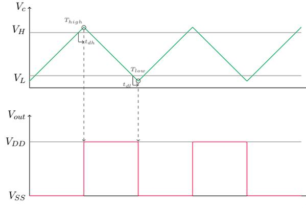
Figure 3.24: Double comparator RO - waveforms
