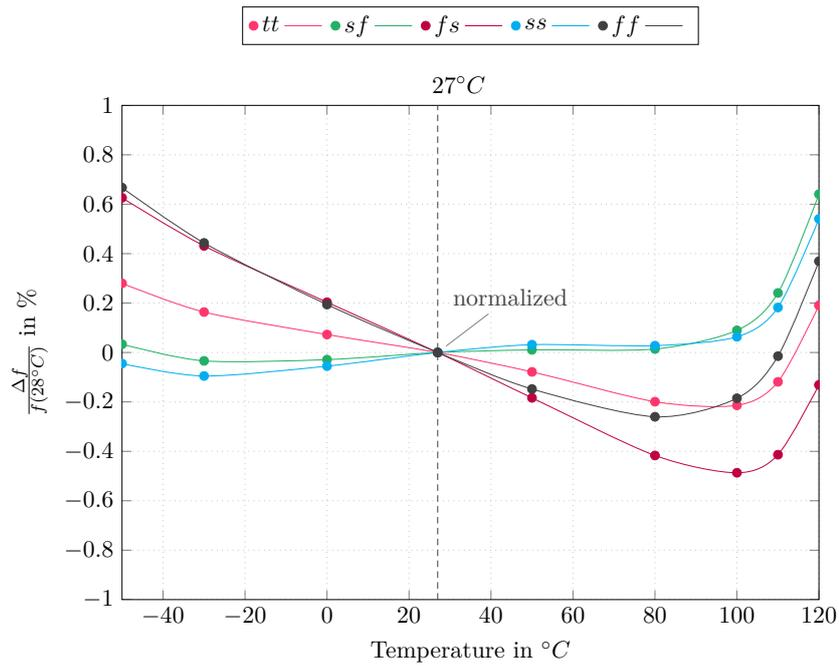
Figure 10.3: Normalized variation of frequency over temperature
