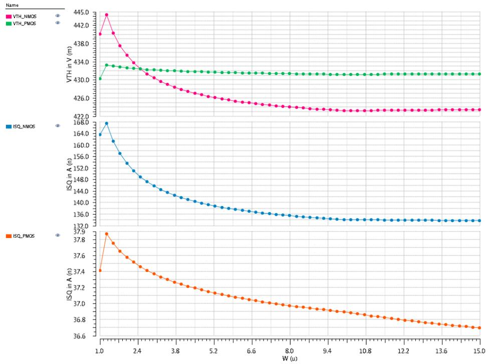
Figure 6.7: Extraction of  $I_{S\Box}$  and  $V_{T0}$  over  $W$ .  $L=10\mu m$ .
