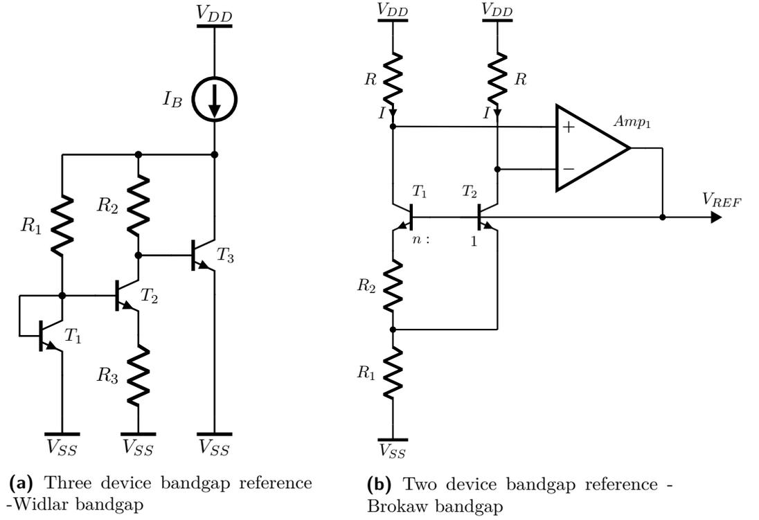
**Figure 5.3:** Bandgap reference design approaches
