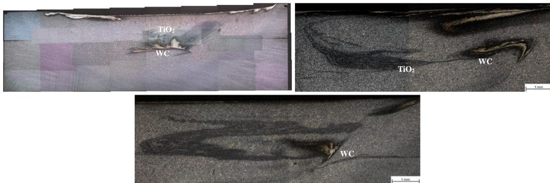
Figure 42 Colored images showing the weld area of sample B (top left), C (top right) and E (below) gold is WC, grey TiO<sub>2</sub>
