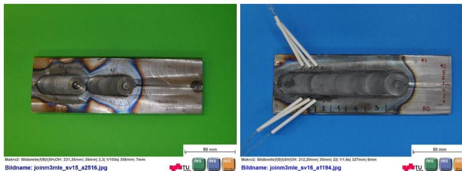
Figure 37 FSW samples E (left, labeled 212a) and D (right, labeled 0)
