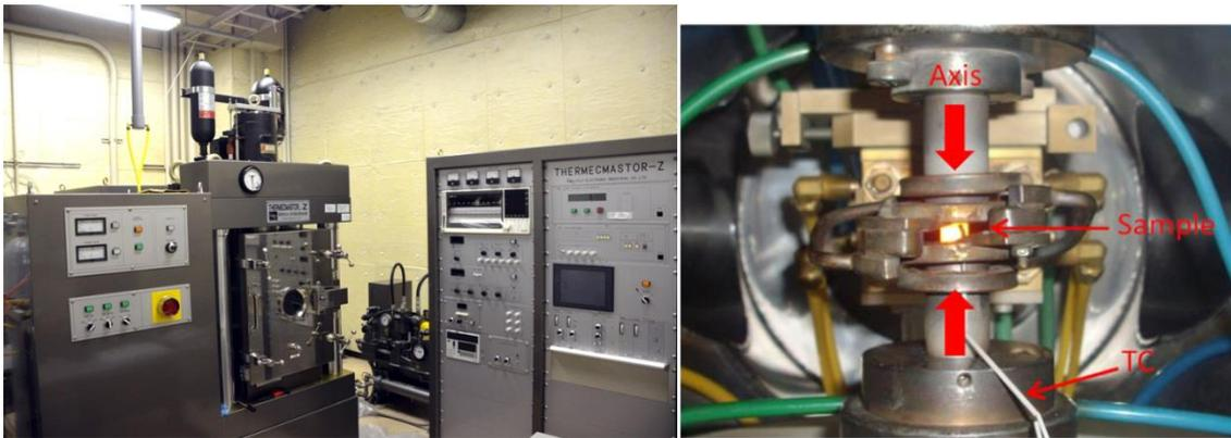
Figure 39 ThermoMaster Z (left) [81] and pressing process (right) similar to the one used in the thesis [84]
