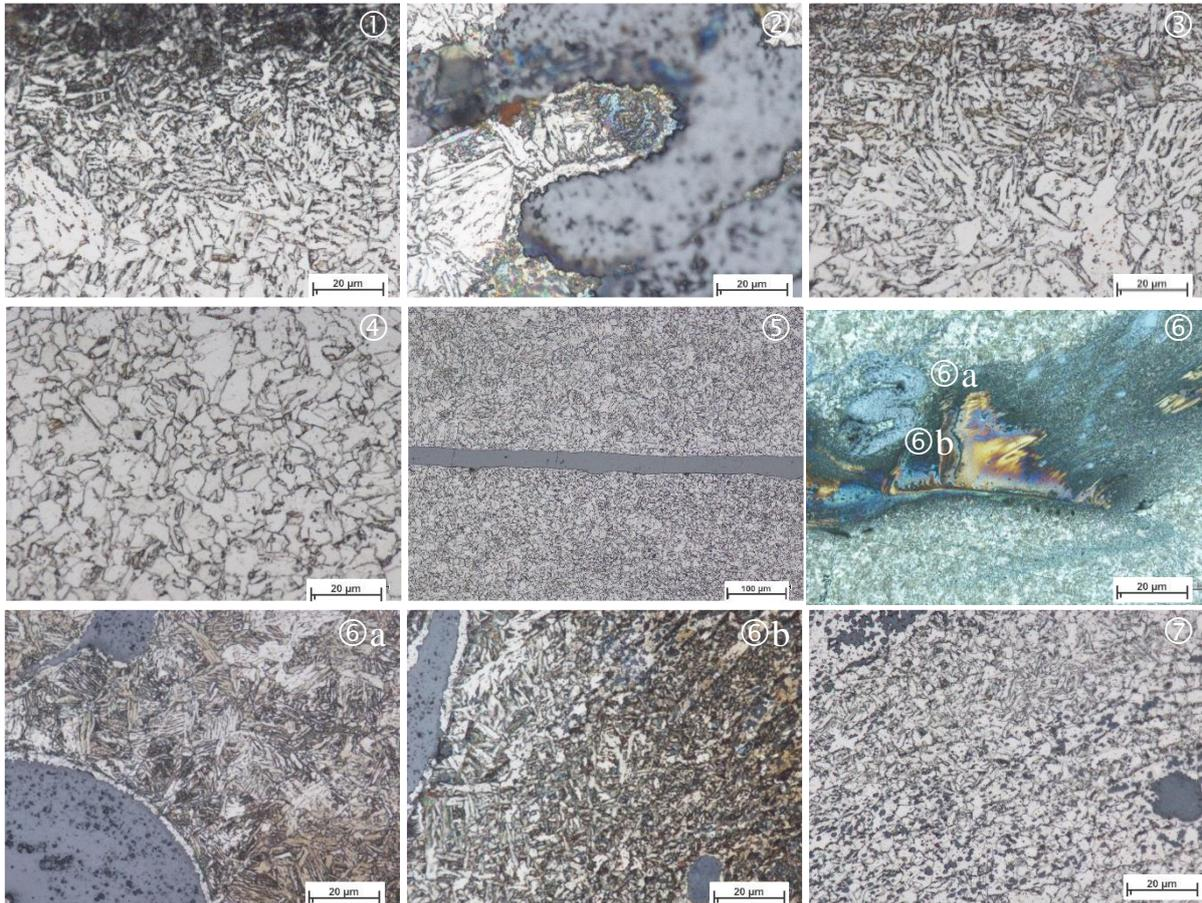
Figure 45 Sample B - LOM microstructure details: ① near surface close to WC abrasion, ② stir zone center and ③ below center, ④ outside TMAZ, ⑤ TiO<sub>2</sub> between plates ⑥, ⑥a) and ⑥b) stir zone center near TiO<sub>2</sub>, ⑦ center right (AS)
