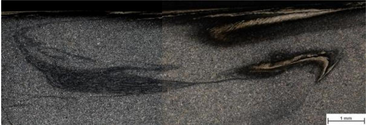
Figure 80 Sample C: Overview center of the weld showing a distinct pattern,  $\text{TiO}_2$  (grey) and tool abrasion (gold color)
