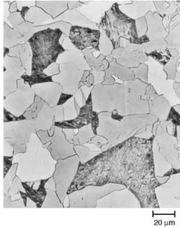
Figure 6 polygonal ferrite(light) and martensite (dark) [25]
