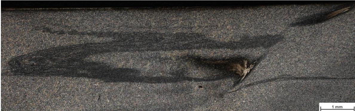
Figure 93 Sample E: Overview center of the weld showing a distinct pattern and tool abrasion (gold color)
