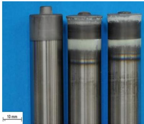
Figure 40 Tool wear during the welding process: initial (left) after 160mm (middle) after one plate (right)
