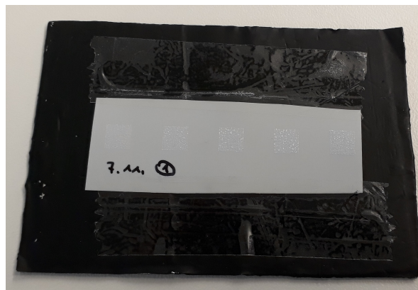
Fig. 3.13.: Sample (Testpattern 1 drop per spot, [11,15,20,25,30] layers) on the blackened aluminum, as it is then measured.
