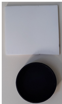
(a) Teflon sheet and lens cover used for measurement of white and black reference spectrum.
