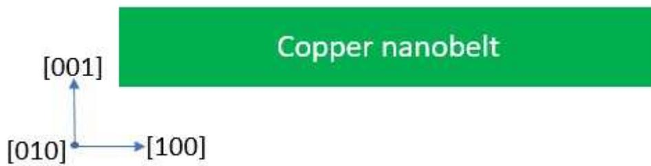
Figure 27 Crystallographic directions in copper nanobelts.
