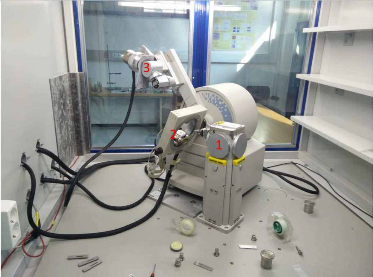
*Figure 16 Measurement chamber of the Philips X'Pert System X-ray diffractometer with indications of the components.*
