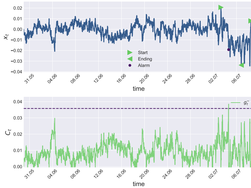
Figure 3.23.: CUSUM test on m_t of pressure sensor HG3835. A leak alarm is triggered on the 4.7. 15:00—2 hours and 40 minutes after the leak was introduced in the system
