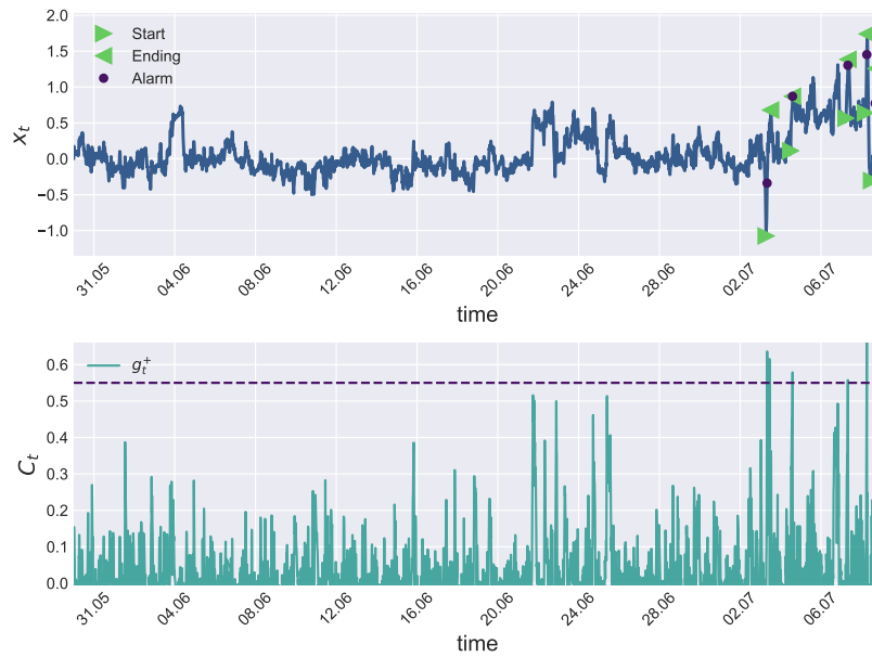
Figure 3.22.: CUSUM test on m_t of the inflow data. A leak alarm is triggered on the 3.7. 08:00 (false alarm) and on the 4.7. 14:15—1 hour and 55 minutes after the leak occurred
