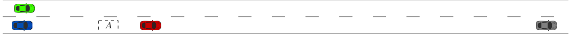
Figure 7.8.: Merging example with one leader (gray) and three following vehicles (colored). The green ego vehicle has to reach position A.
