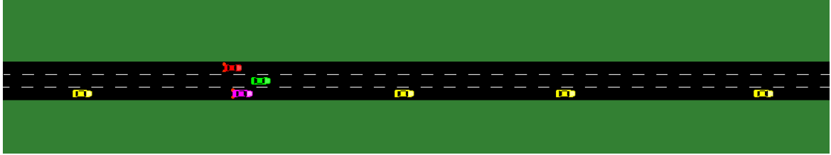
Figure 3.21.: Simulation studies of the MWC visualized in SUMO after t_3 (ego vehicle in red)
