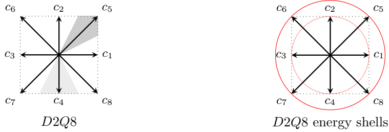
Figure 3.10.: Regions of influence (marked grey) for the D2Q8 lattice based on [19] and corresponding energy shells (marked red)
