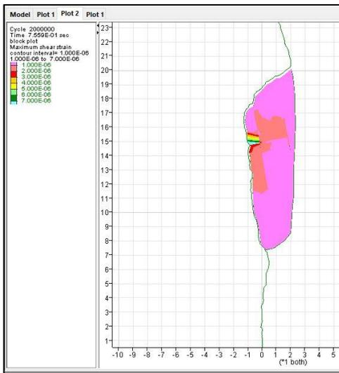
Fig. 93:  $jkn = 1E12, jks = 1E12, c = 0, \text{step } 2E6$
