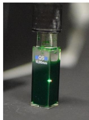
Figure 44. Green fluorescence determined by excitation with a laser diode at 635 nm (*polymer I*, 1,4-dioxane).
