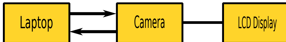
Figure 5.18.: Setup for vignetting correction.
