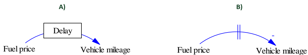
Figure 32: Possible notations for system delays in a Causal Loop Diagram
