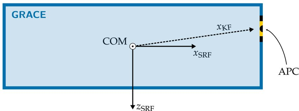
Figure 4.2: Exaggerated depiction of the misalignment of the calibrated KBR antenna phase centre with the SRF x-axis (side view).
