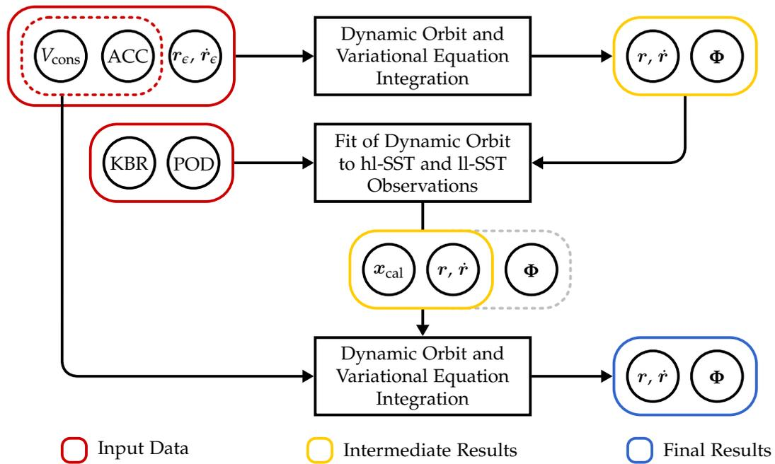
**Figure 6.4:** Data flow in ITSG-Grace2016 dynamic orbit integration for one spacecraft.  $V_{\text{cons}}$  are the background models from which the accelerations due to conservative forces are derived, as given in table 6.1.  $\Phi$  is the state transition matrix of the variational equations.  $x_{\text{cal}}$  are the co-estimated calibration parameters for the accelerometer.
