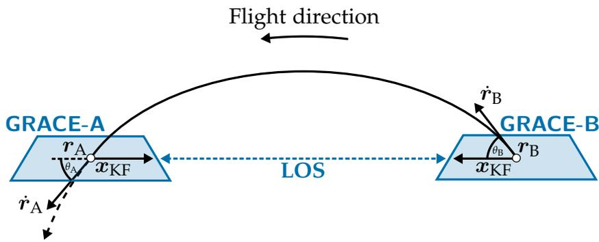
Figure 4.4: In-orbit formation of the GRACE satellites in science mode with pitch bias  $\theta_{A/B}$ . Adapted from Kirschner, Montenbruck, and Bettadpur (2001).
