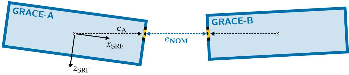
Figure 8.2: Orientation of spacecraft in nominal attitude with APC vector
