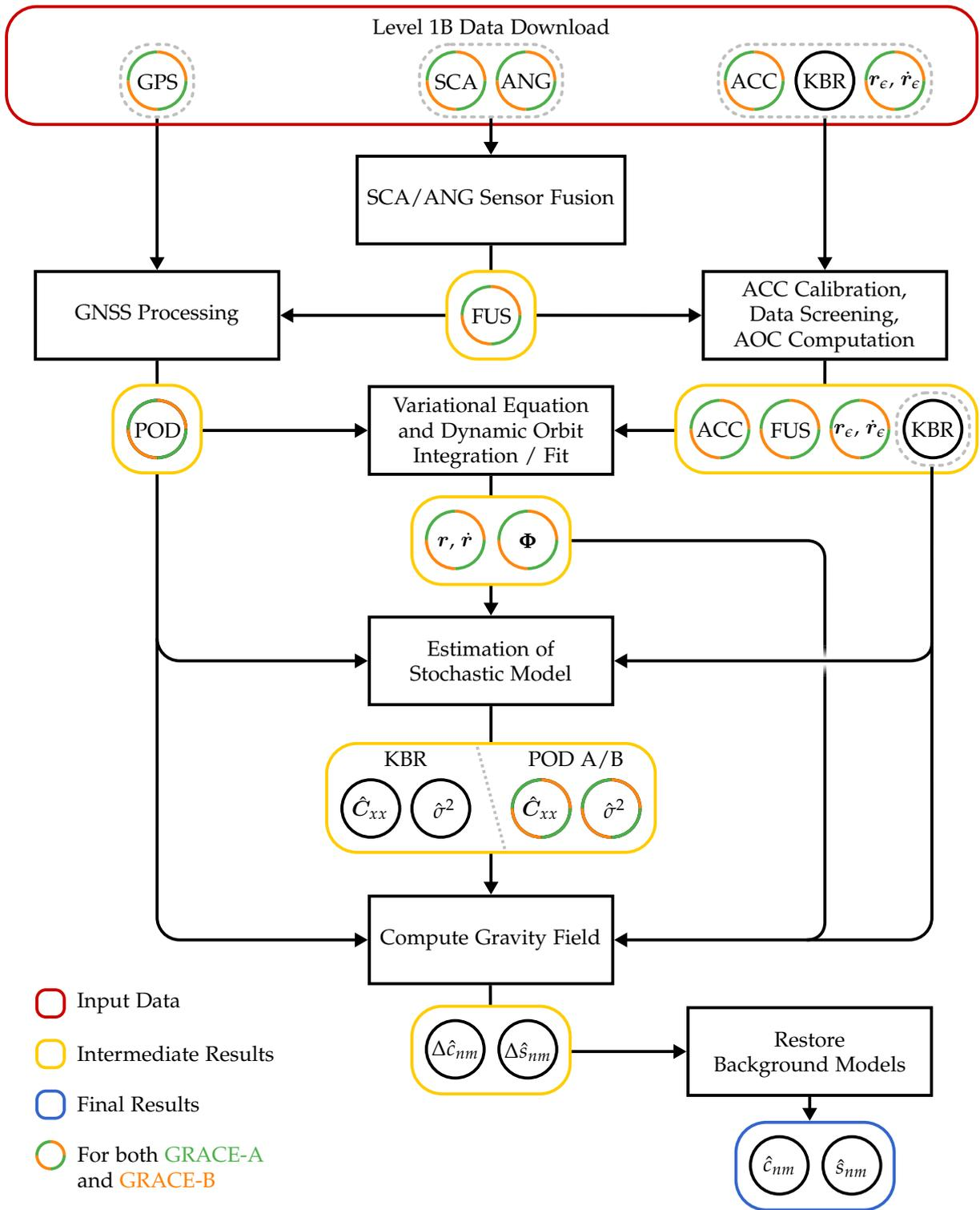
Figure 6.1: Schematic for ITSG-Grace2016 level 1B to level 2 data processing.  $\Phi$  is the state transition matrix of the variational equations.  $x_{cal}$  are the co-estimated calibration parameters for the accelerometer.
