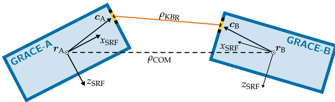
Figure 4.3: Observation geometry of the GRACE KBR measurement.
