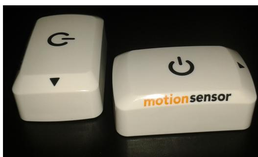
Figure 3.1.: Tyromotions IMU-based Motionsensor.
