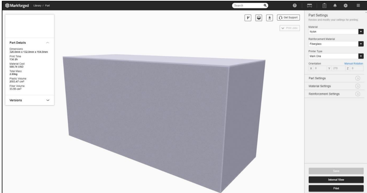
Figure 5-3: Maximal build volume of the MarkForged Mark One™ 3D printer
