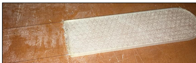
Figure 5-15 Printed prototype PT02 with an integrated ORMOCER® coated optical fiber
