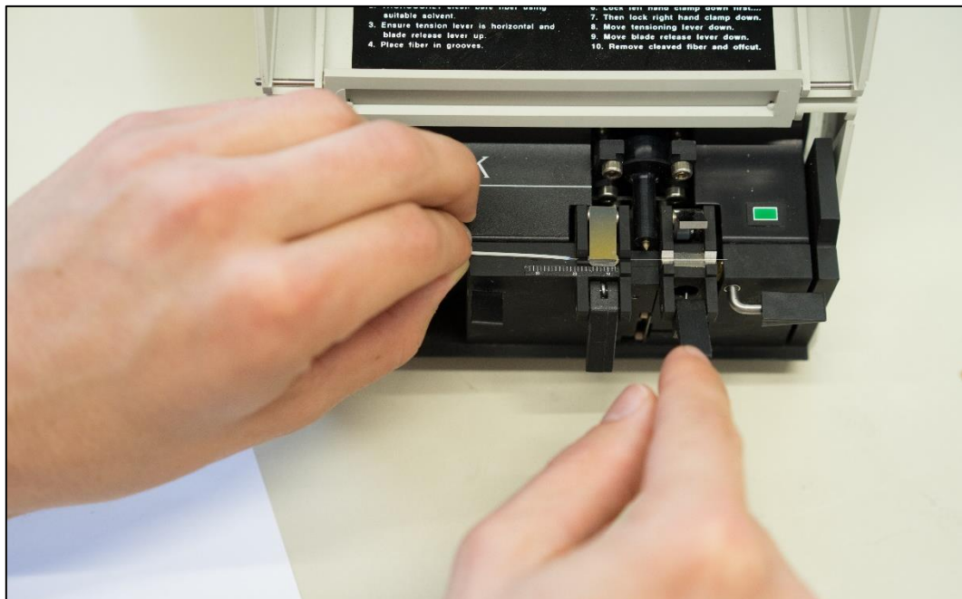
Figure 5-11: Cleaving the bare optical fiber of the pigtail
