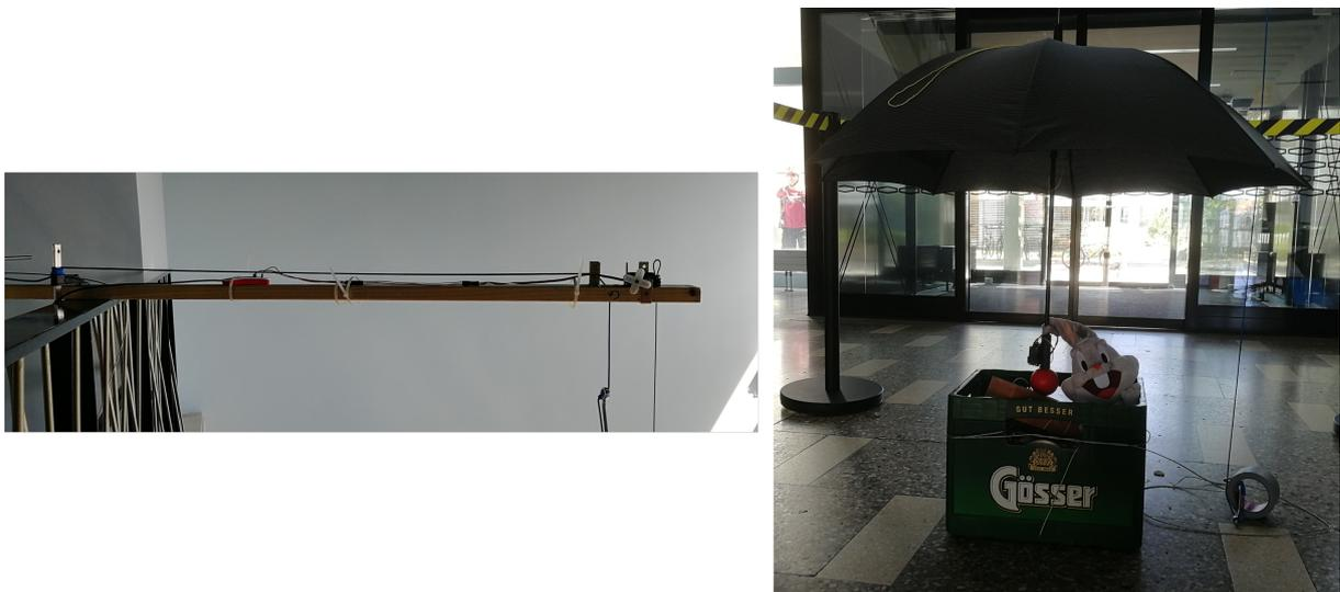
Figure 2.2: (left) Wooden brick which is attached to the handrail at the 5th floor. The steel cable is fixated on the right part of it. (right) steel cable fixated with the help of a box filled with stones and the umbrella which was used as parachute.
