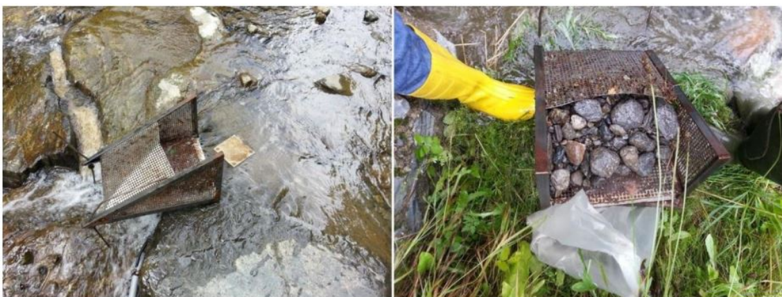
Figure 3.25: Installed SIS and bed load sampler (Spreitzer (2014))
