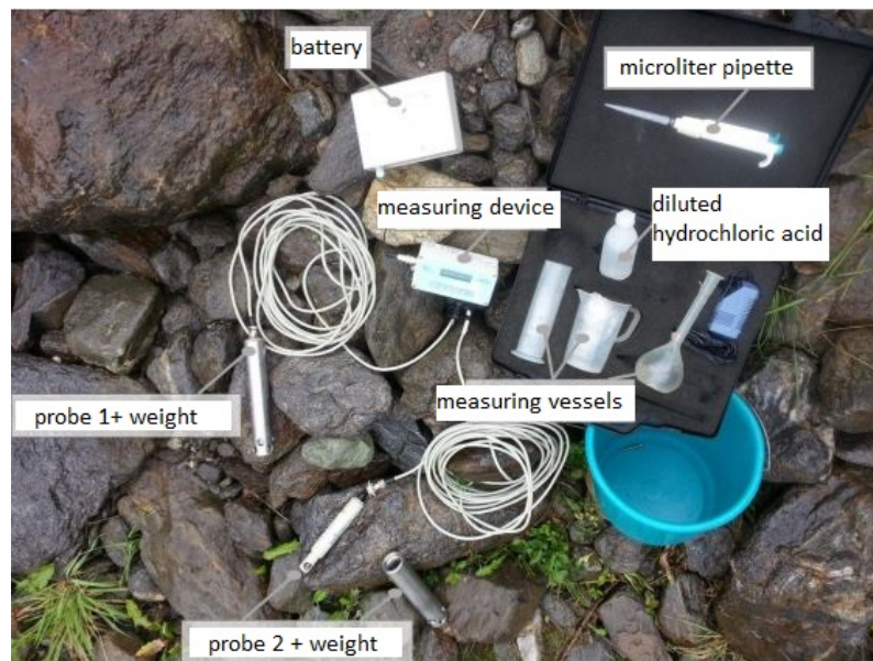
Figure 3.7: Saltracer equipment (Spreitzer (2014) modified)
