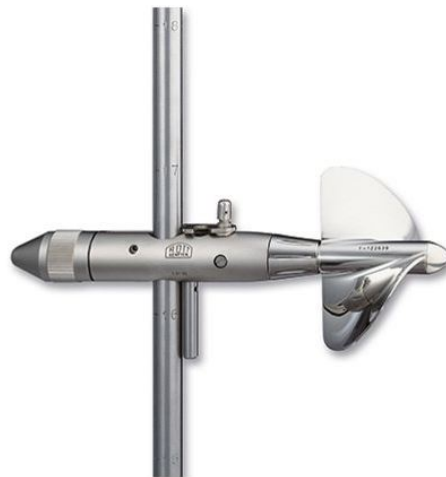
Figure 3.9: Current meter (OTT Hydromet GmbH (2018))
