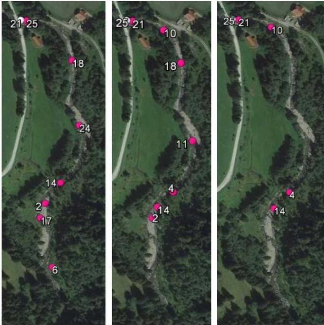
Figure 3.23: Transport distance of tracer stones for 22.July-29.September 2016 (Langer, Stoisser (2016))
