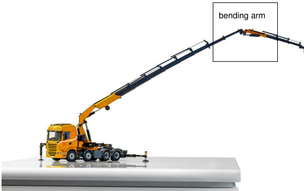
Figure 16 Additional bending arm 183
