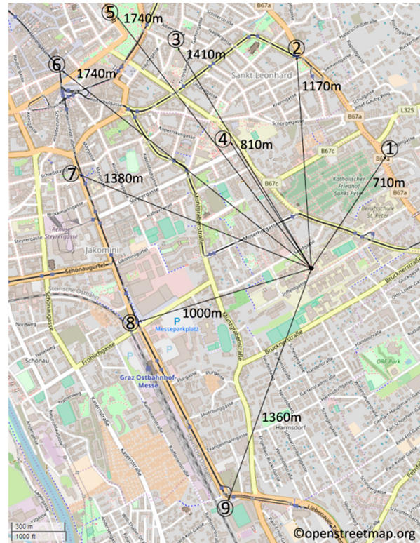
Fig. 2. Map of the distance measurement showing sink, node positions (1–9) and the distance between them
