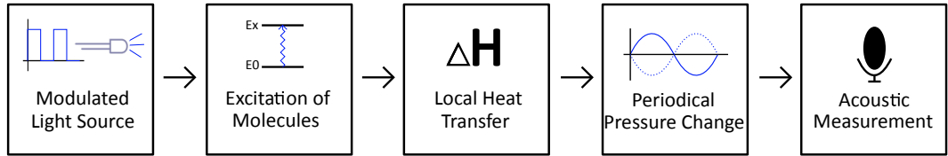
Figure 2.1.: Block diagram of photoacoustic spectroscopy. A modulated light source is used to excite molecules to enter higher energy states. This absorbed energy is subsequently transferred into kinetic energy. The movement of molecules causes inelastic collisions, which trigger a periodic heat change and consequently a periodical pressure change. This pressure change can be measured by an acoustic sensitive device.
